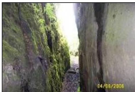
**Figure 1.** (Left) Odin Cave and Odin Mine, note the mine waste tips on the lower right of the photograph. (Right) The worked-out Odin mineral vein with mineralised, horizontal slickensides on the hanging wall.
