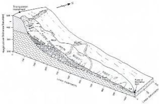
**Figure 4.** The main features of the Mam Tor landslide. Distances in metres, height in metres above Ordnance Datum (modified after Varnes 1978, in Cripps & Hird 1992).
