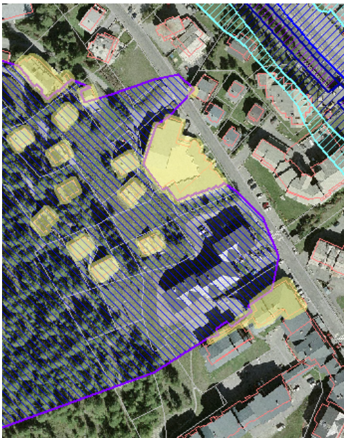
Figure 4. Identification of exposed buildings to avalanche corridor
