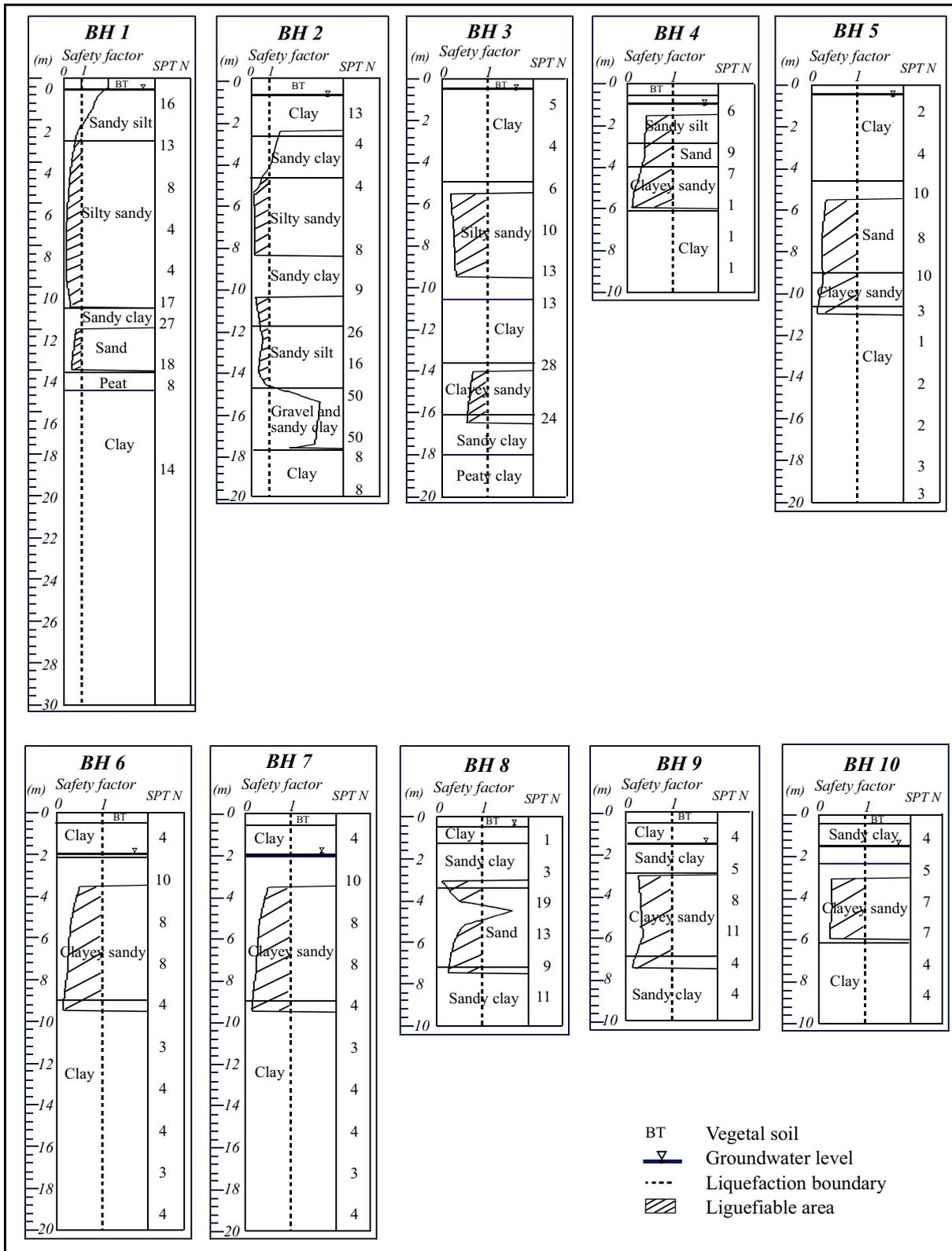
Figure 6. Logs, SPT N value and liquefiable area
