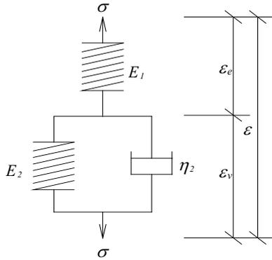
Figure 1. Three-element visco-elastic model
