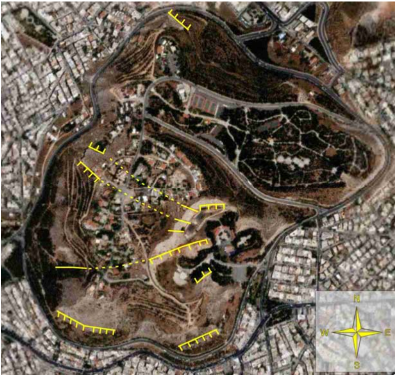
Figure 1. Aerial photograph of Tourkovounia hill. The “Attiko Alsos” park is located in the SE section of the hill. This park consists of a public garden, an open air theatre, a volley-ball and a basket-ball field, a coffee-bar and an extensive parking area. This figure presents some of the normal faults which, in spite of the intensive alteration of the morphology, are visible in the aerial photograph. The covered extensions of those faults go across the built-up area located on the top of the hill and under the foundations of the houses.
