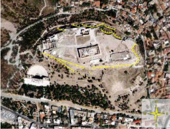
Figure 4. Aerial photograph of Acropolis hill. Major tectonic fractures – normal faults of ENE-WSW to SE-NW direction traced on the photograph.
