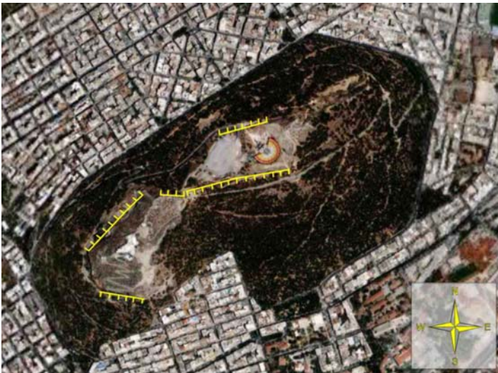
Figure 5. Aerial photograph of Likavitos hill. Major tectonic fractures – normal faults of ENE-WSW to SE-NW direction traced on the photograph.
