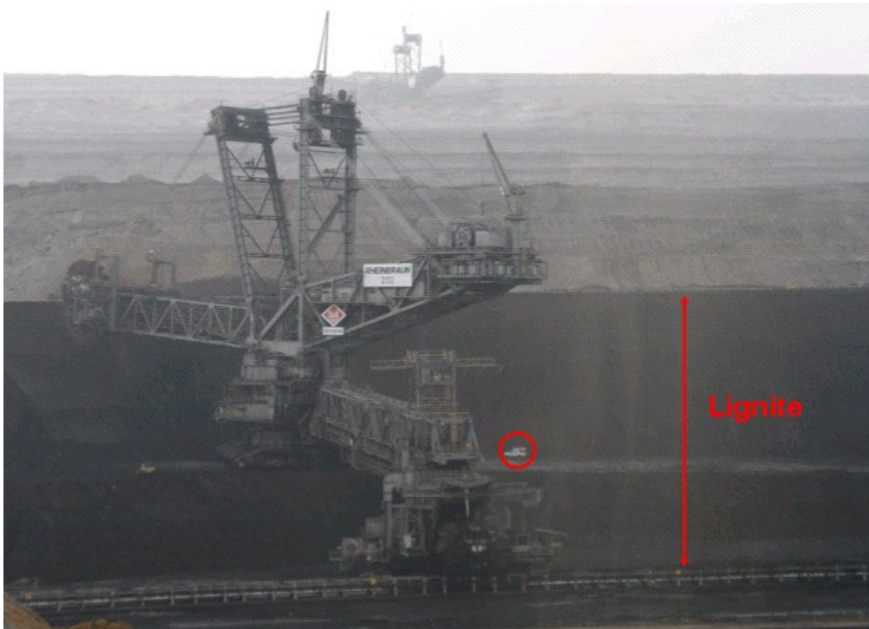
Figure 5. The circle marks a Landrover Defender for scale. The bucket wheel excavator (here operating on a bench 14 m above the conveyor belt) is 90 m high.
