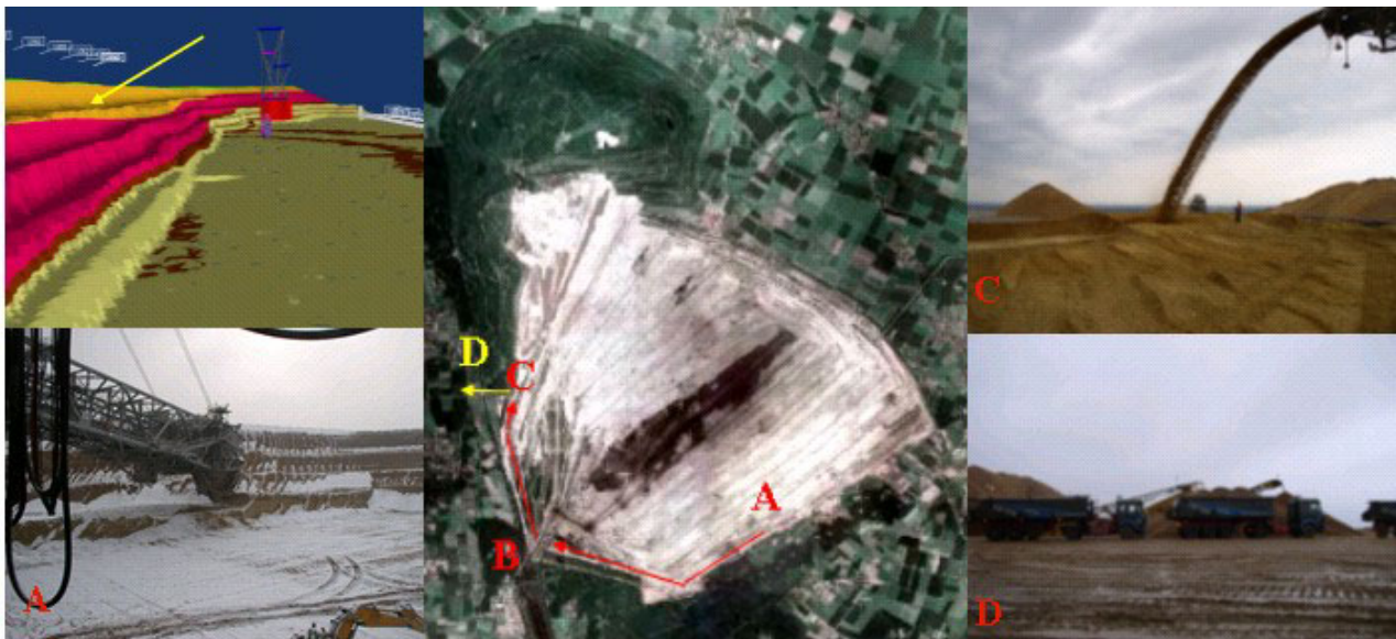
Figure 11. Top left: In the subsurface model the gravel layers (orange) can be identified. Bottom left: The bucket wheel excavator is moving towards this material. Middle: The gravel excavated by the bucket wheel excavator at e.g. A is transported via conveyor belts to the conveyor belt junction at B. From here the material is transported to stackers at C. Top right: a stacker depositing gravel. Bottom right (D): Stacking gravel is processed further by sieving. The haulers deliver the gravel to the customer.
