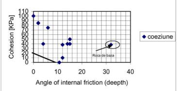
The residual values of the shearing parameters are represented by means of a straight line with the coordinates  $(9^\circ, 20 \text{ kPa})$ , resulting both from the laboratory tests and from the calculation of the stability limit of the slope. By examining them we notice easily that a series of values are situated near the high risk-limit in respect of the stability of the slope. From the distribution of the plasticity index with the depth we find the distribution of the variation of the
