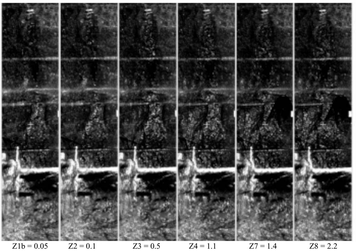
Figure 8. Water leakages with different flows shown as a grey-scale image
