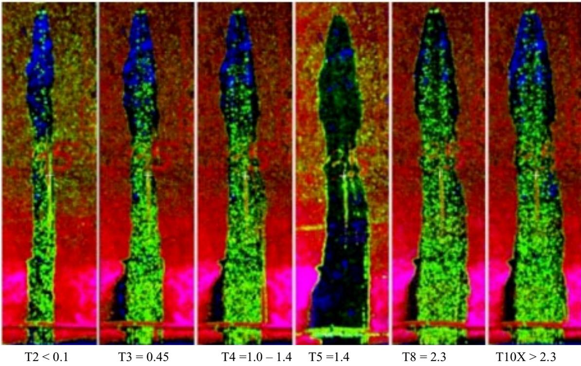
Figure 7. Different water leakages shown as a pseudo-colour image of the TBM tunnel wall
