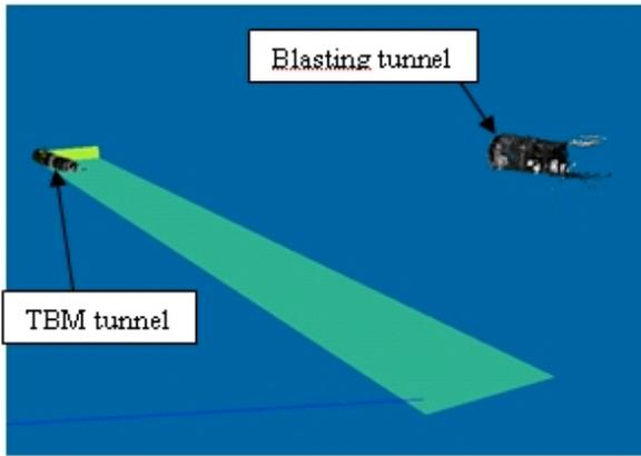
**Figure 3.** Two scanned tunnels registered in the same co-ordinate system
