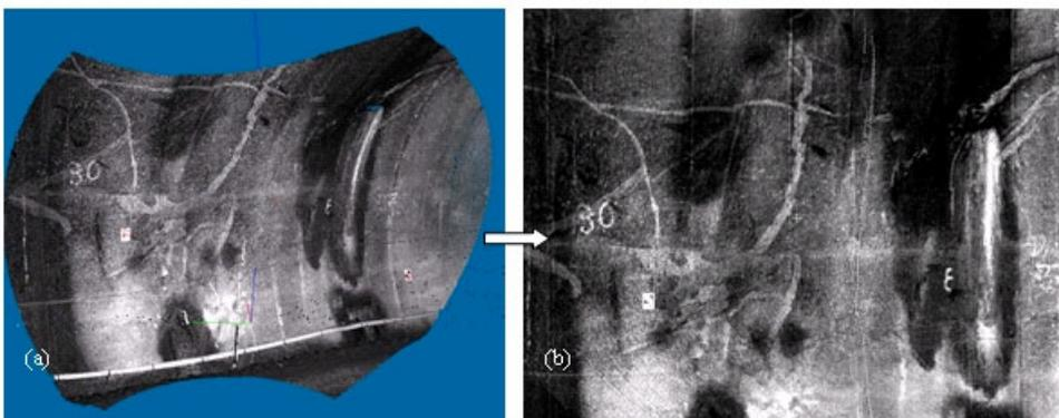
**Figure 4** Convert from 3D laser image (a) to 2D ortho-projected laser image (b)
