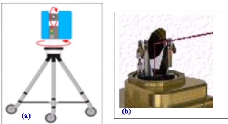
**Figure 1.** Leica HDS4500 laser scanner (a) and its scanning head (b)
