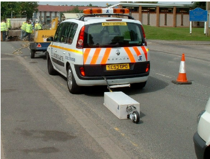
Figure 3. GPR survey vehicle, with antennae housing in towing position
