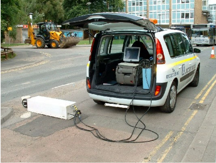
Figure 4. Transverse survey across road. The display screen is visible inside the survey vehicle, with SIR-10H unit to its right (connected to the antennae box by three cables).
