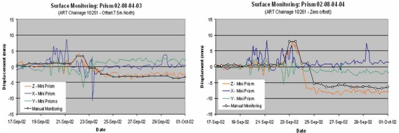
Figure 9. Comparison of manual precise levelling and data from automated mini prism survey
