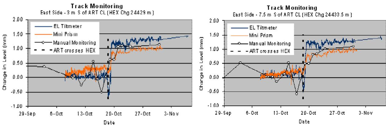
**Figure 15.** Comparison of HEX vertical track movement at (a) 3m south, (b) 7.5m south of ART centreline
