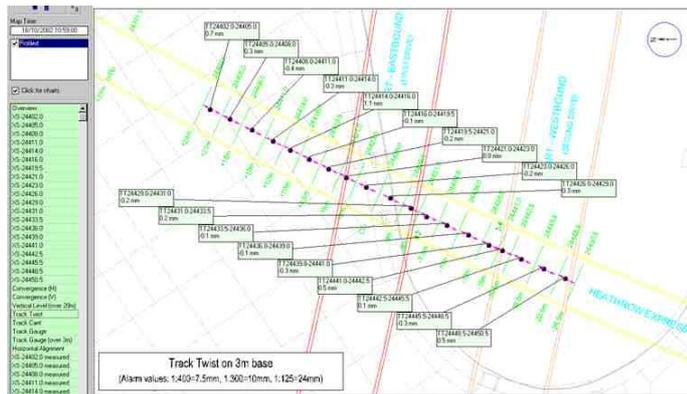
**Figure 14.** Data interface from I-Site® software showing locations of monitoring arrays within the HEX tunnel
