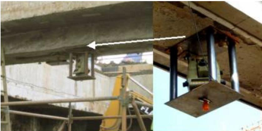
**Figure 4.** Leica TCA 1800 total station mounted in the TBM chamber
