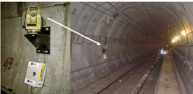
Figure 13. Automated total station located within HEX tunnel
