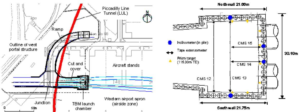
Figure 3. (a) West Portal location plan, (b) TBM launch chamber plan (CMS – convergence measurement section)
