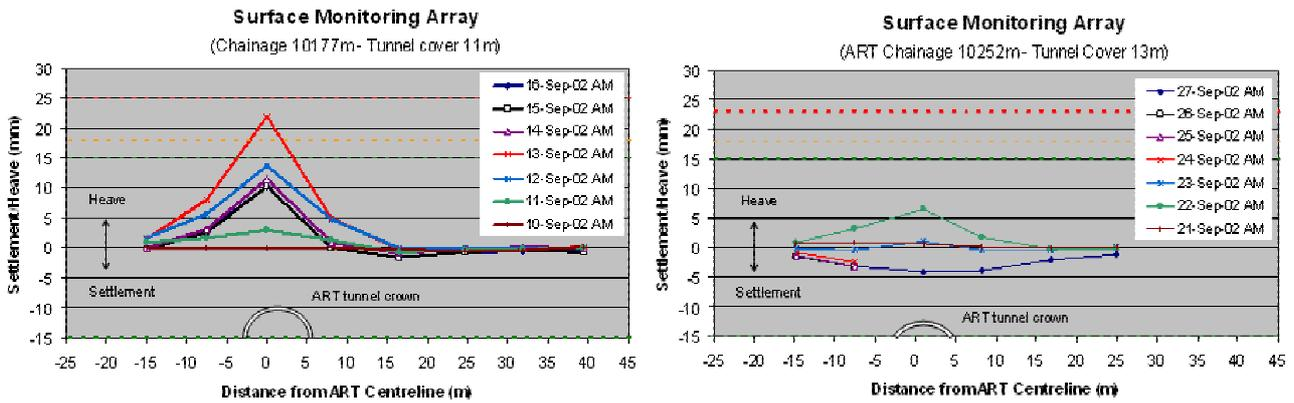
Figure 8. Tunnel induced ground surface movement at (a) ART Chainage 10177, and (b) ART Chainage 10252
