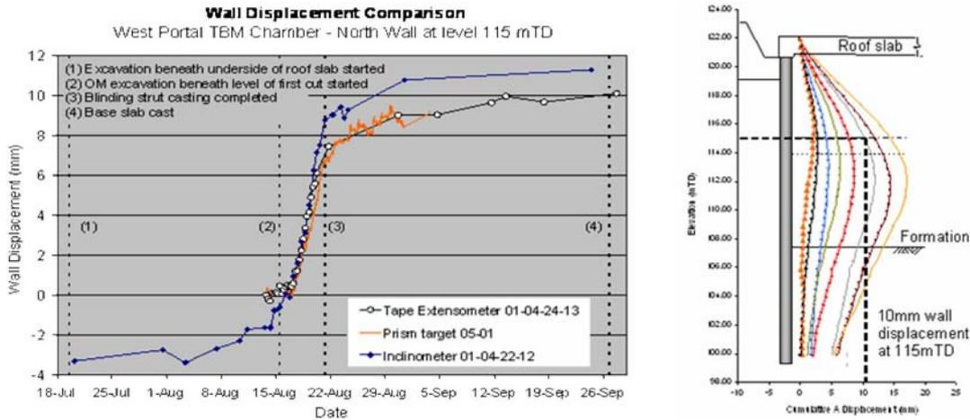
Figure 5. Comparison of TBM chamber monitoring data & inclinometer profile (north wall)
