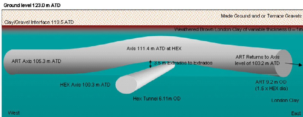
Figure 11. Schematic drawing of ART crossing existing HEX tunnel (not to scale)
