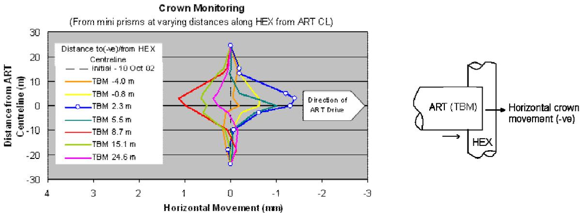
Figure 17. Horizontal movement of the HEX crown at various distances along the tunnel from the ART centreline
