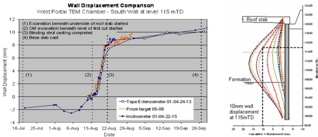
Figure 6. Comparison of TBM chamber monitoring data & inclinometer profile (south wall)
