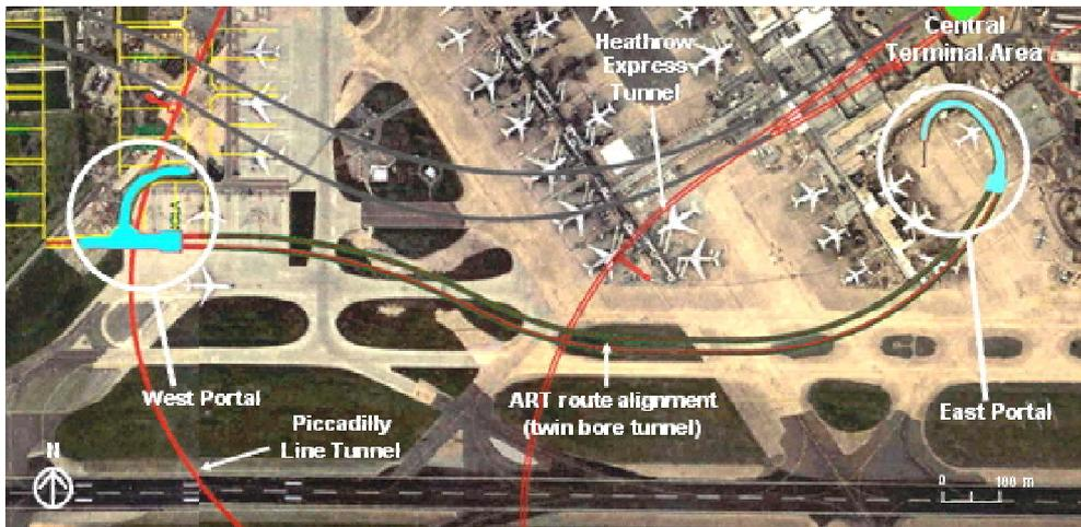
Figure 1. Location plan of the Airside Road Tunnel (ART) at Heathrow Airport
