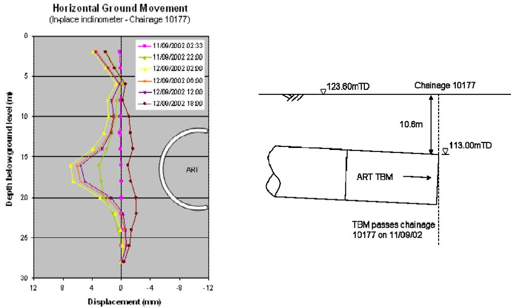
Figure 10. Horizontal ground movement from in-place inclinometers at chainage 10177 (TBM pass on 11 Sep 2002)
