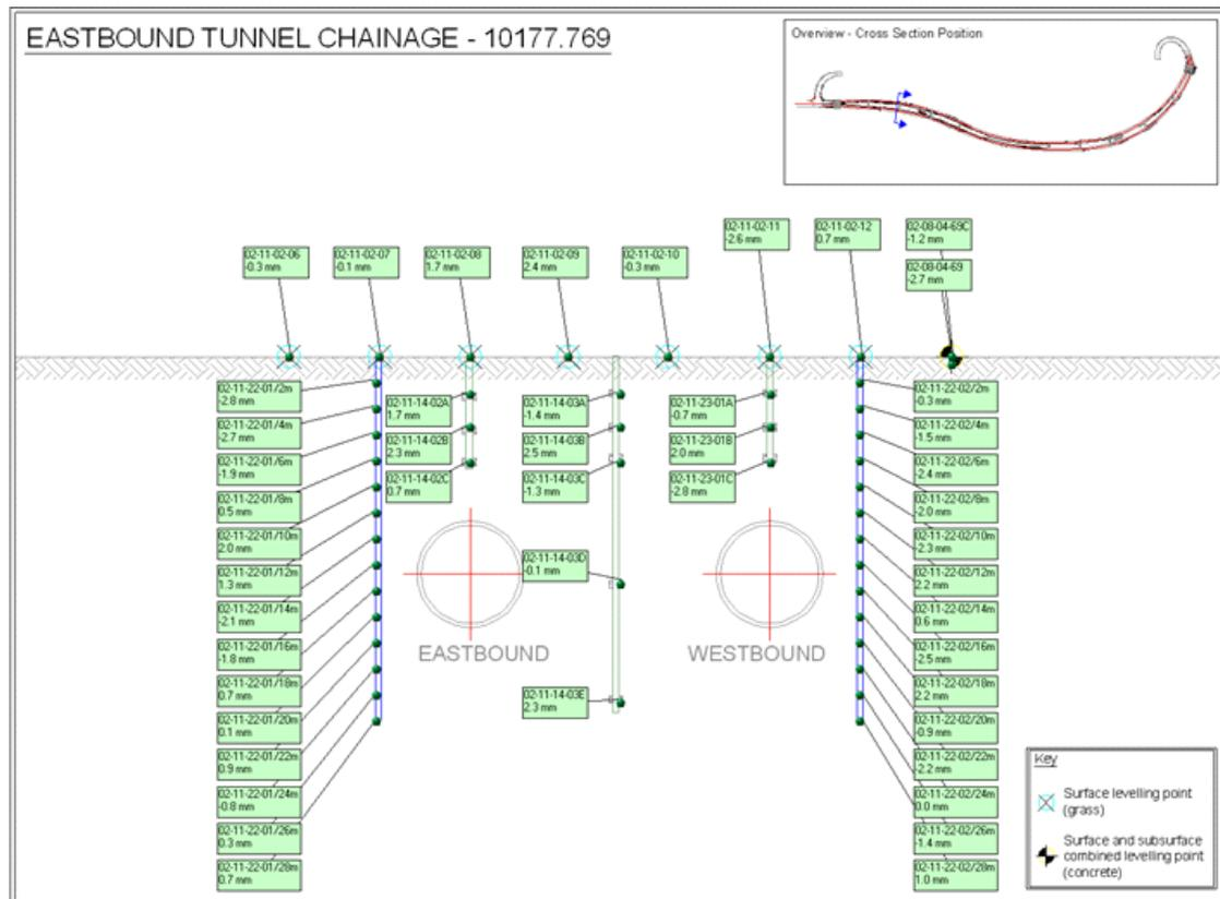
Figure 7. Automated deep section monitoring array (ART Chainage 10177)
