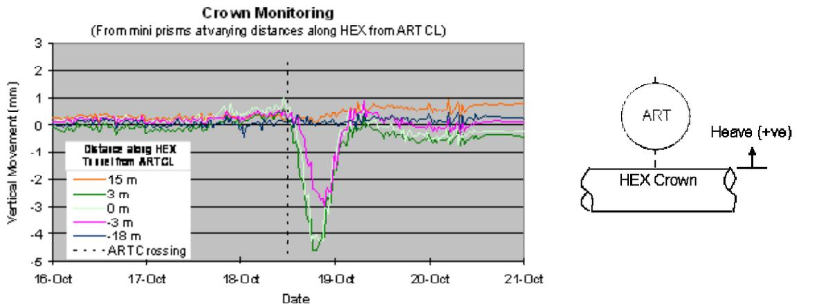
Figure 16. Vertical movement of the HEX crown at various distances along the tunnel from the ART centreline
