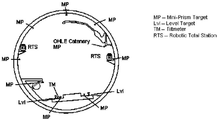
Figure 12. HEX tunnel instrumentation
