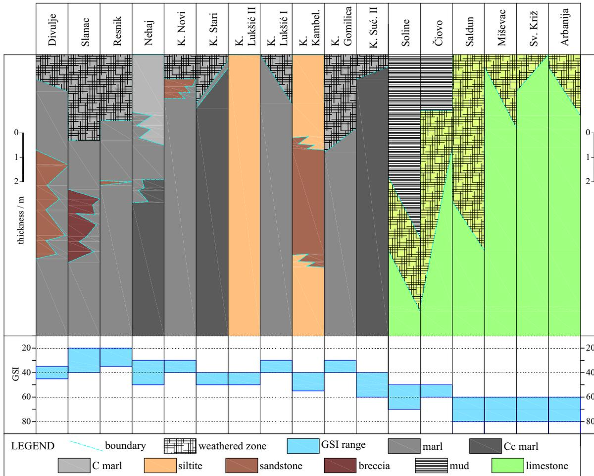
**Figure 4.** Schematic and simplified cross-sections (excluding anthropogenic layers) through the flysch and limestone, showing the weathered zone and clastic components of the flysch. Geological Strength Index (GSI) values are for fresh or slightly weathered bedrock.
