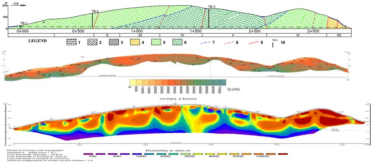
**Figure 7.** a.) Geological profile with engineering-geological units (legend is the same as in Figure 6). b.) Seismic refraction profile. c.) Geoelectrical tomographic profile.
