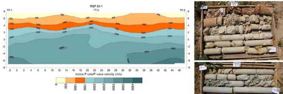
Figure 3. Seismic refraction profile and borehole core at the location of the Divulje pumping station.
