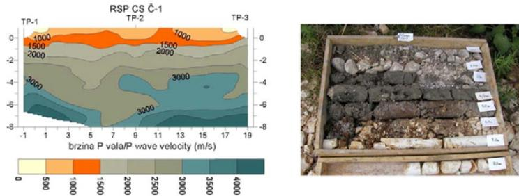
Figure 5. Seismic refraction profile and borehole core at the Ciovo pumping station location.
