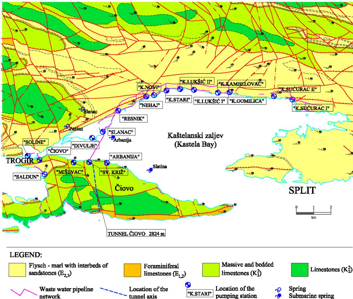
Figure 2. Geological map of the region (after Marincic et al. 1973), and the Kastela Bay proposed sewage system.
