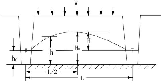
**Figure 2.** The lay of blind channel
