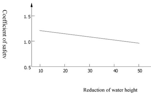
Figure 1. The relation between reduction of water height and coefficient of safety of slope
