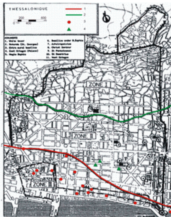
Figure 2. Map of the historical centre of Thessaloniki (after Tsotsos et al. 1988). 1. Natural coastline, 2. Zone I – II boundary, 3. Boreholes where organic silt was found, 4. Boreholes where organic silt was not found.
