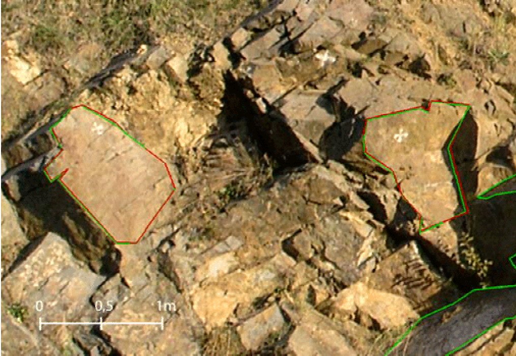
Figure 6. Measurement of the rock blocks edges by the method of digital photogrammetry (red line – position in 2004, green line – position in 2005)
