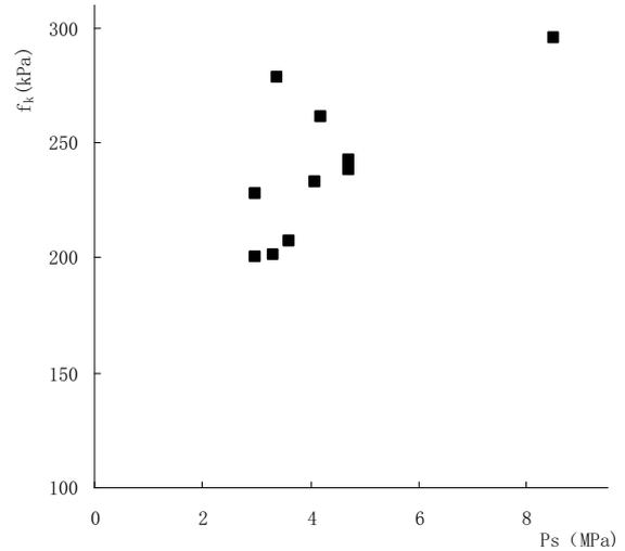
**Figure 6.** Relationship between the bearing capacity of deep soil layer ( $f_k$ ) and CPT ( $P_s$ )
