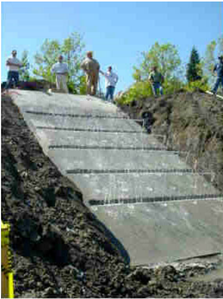
Figure 5. Concrete slab at test site outfitted with an array of plate pile sleeves and subsurface irrigation lines
