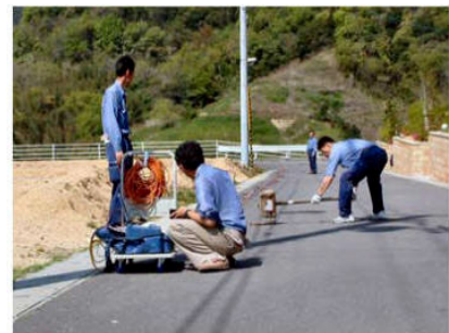
Figure 2. Operation of the surface wave prospecting
