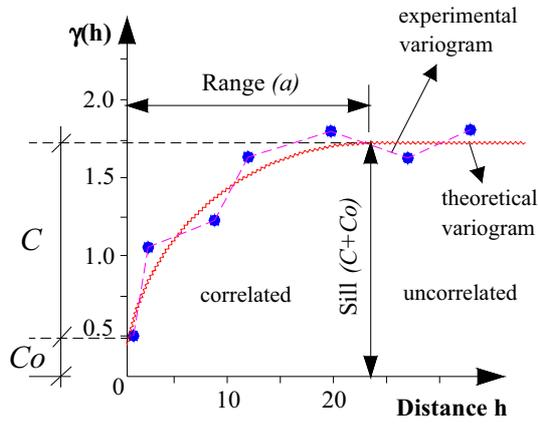
**Figure 2.** Theoretical variogram fitted to an experimental variogram
