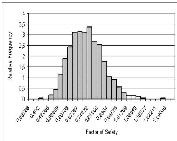
**Figure 6.** Distribution of the slope 2 factor of safety histogram. The factor of safety was determined from the mean  $\phi$  and 40% of the TC filled with water (normal distribution). The grey bars at the left of the distribution represent situations with factor of safety less than 1.0
