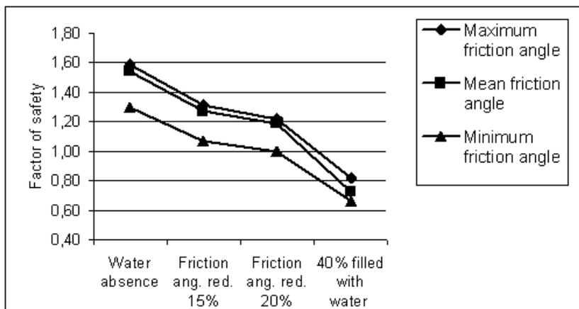
Figure 2. Variation of the FS values of slope 2 for different water conditions and friction angles
