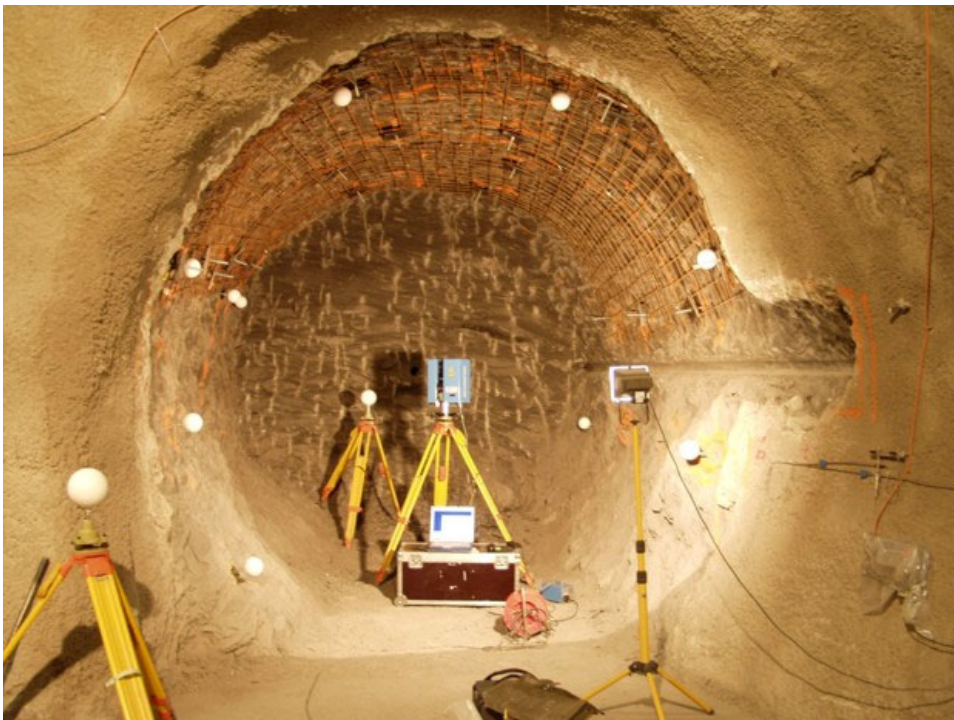
Figure 1. Imager 5003 laser scanner of Zoller+Fröhlich and overview of the excavated experimental tunnel
