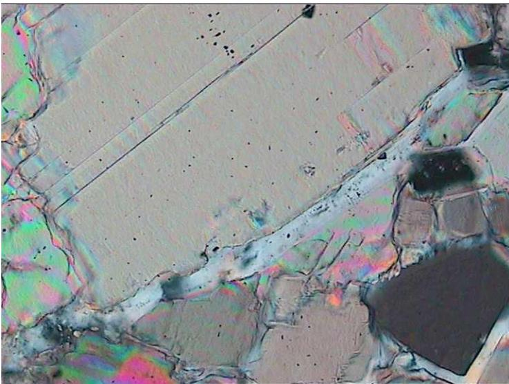
**Figure 7.** Thin section image of the Haselgebirge sample with large anhydrite crystals. Crossed nicols, picture width approx. 0.65 mm.
