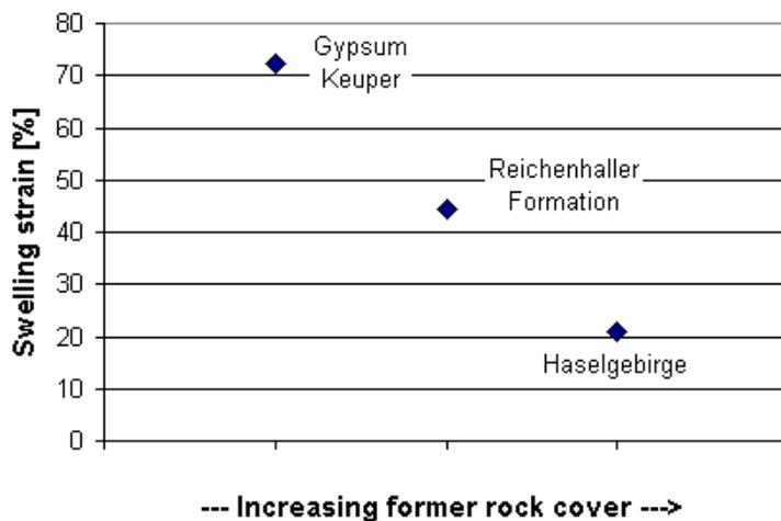
**Figure 5.** Decreasing swelling capacity against increasing former rock cover after around 1 year of swelling. The swelling in percent is related to the sample height at the beginning of the test.
