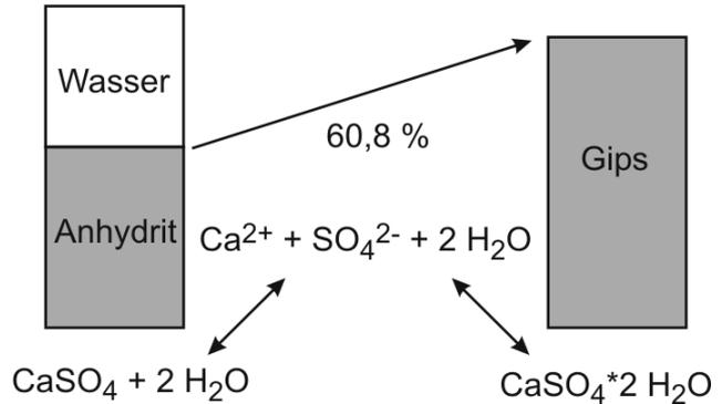
**Figure 3.** Chemical and physical basics of the of anhydrite-gypsum conversion. The reaction goes through a solution and crystallisation phase (modified after Amstad & Kovari 2001).
