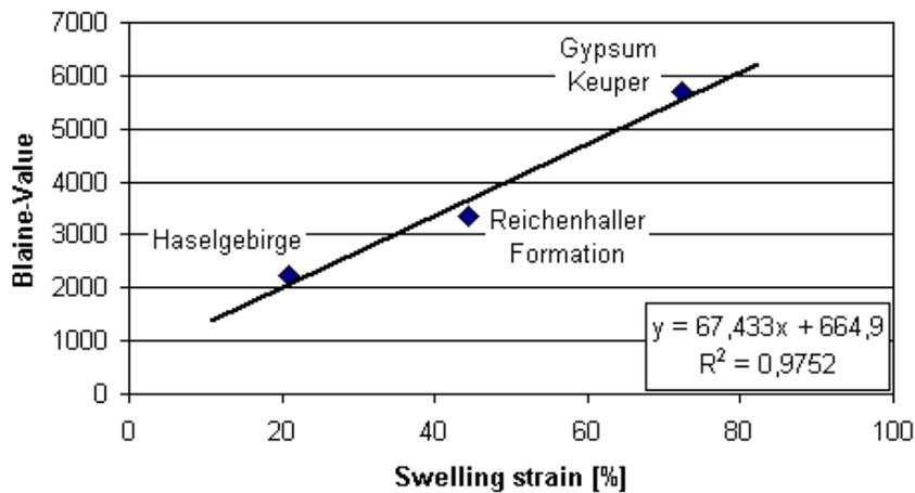
**Figure 11.** Linear correlation between Blaine-Value (specific surface after DIN 196-6 (1990)) and swelling capacity (from the powder swelling test according to Thuro 1993).
