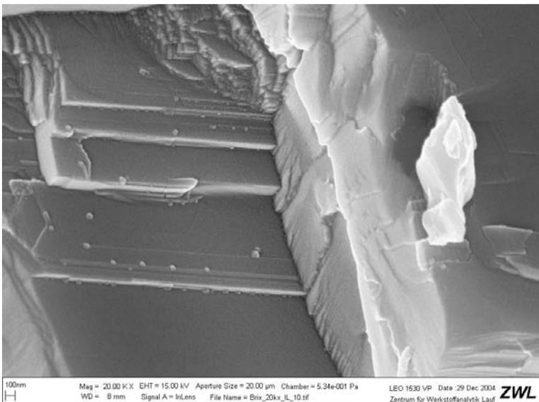
**Figure 9.** SEM image of the Reichenhaller formation anhydrite sample. The material looks very compact and impervious. Picture width approx. 5000 nm.
