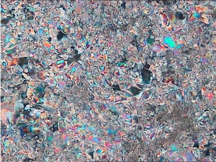
**Figure 6.** Thin section image of the Gypsum Keuper sample with small anhydrite crystals. Crossed nicols, picture width approx. 0.65 mm.
