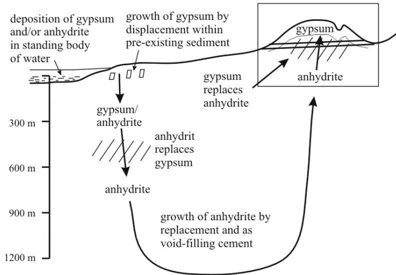
**Figure 1.** Schematic diagram illustrating gypsum-anhydrite-gypsum cycle (according to Murray 1964). The rectangle on the upper right side is shown in detail in Figure 2.
