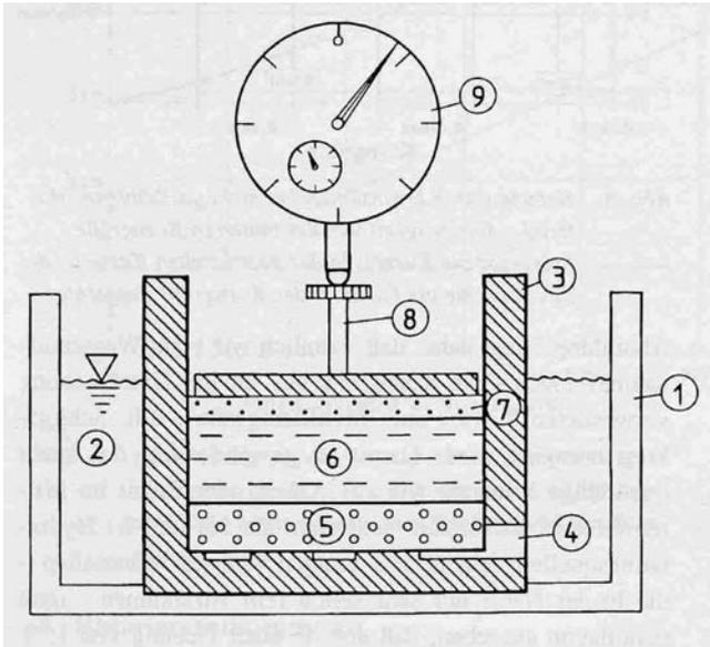
**Figure 4.** Drawing showing the test setup ("Oedometerzelle") for the powder swelling test. 1=water tray, 2=water, 3=swelling cell, 4=drainage hole, 5=lower porous plate, 6=sample, 7=upper porous plate, 8=cap, 9=dial gauge (according to Thuro 1993).
