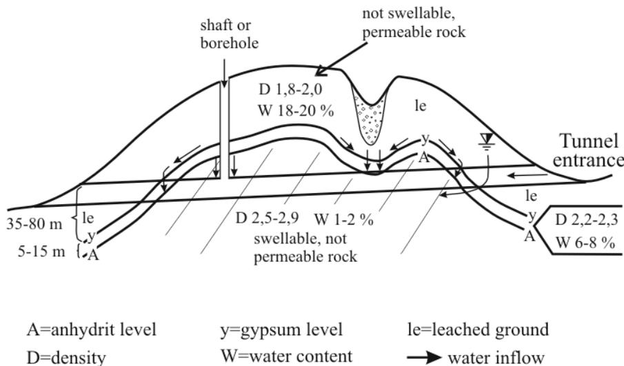
**Figure 2.** Rock characteristics in a sulphate containing rock mass. Also shown are areas of potential water inflow into a tunnel tube (Schematic cross section, modified according to Spaun 1979 and Amstad & Kovari 2001).
