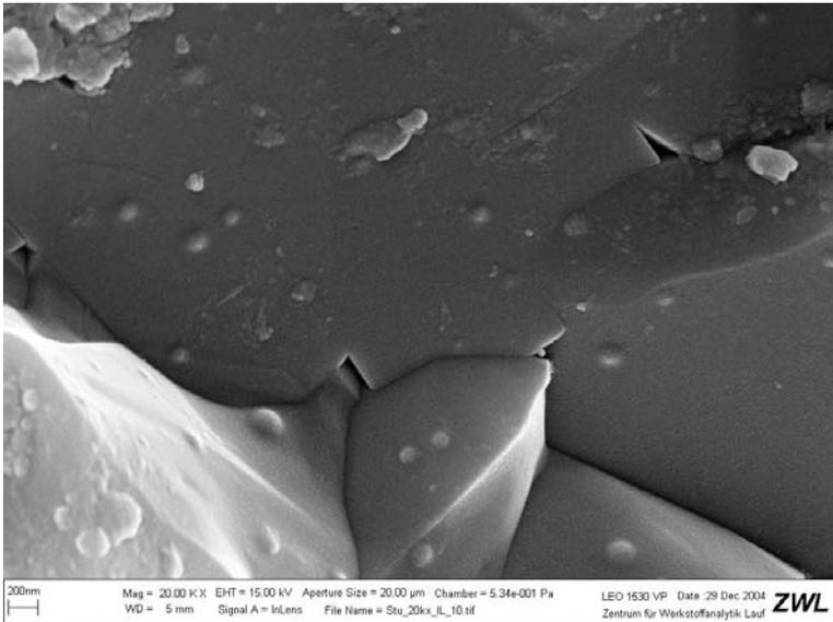
**Figure 8.** SEM image of the Gypsum Keuper anhydrite sample. Please notice the pores between the single crystals. Picture width approx. 5000 nm.
