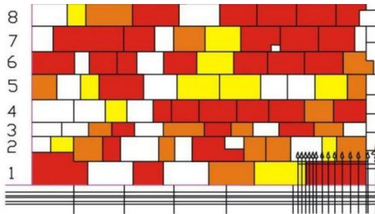
**Figure 11.** Decay classification, based on Figure 10. The different colours of the blocks present different kinds of restoration measures. They are dependent on the factor of time. Explanation of the colours: white (no procedure necessary), yellow (no to minimum action required), orange (middle action for flaking and granular disintegration into sand over stable grounds), red (partial washed surfaces).
