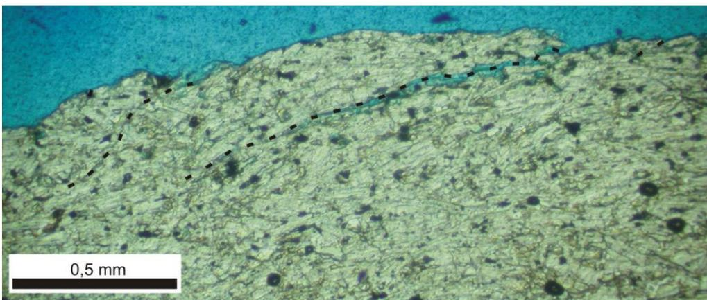
**Figure 12.** Thin section of trachyte embedded in colour resin under vacuum. After chiseller like treatment micro-cracks can be seen on the surface of the trachyte which are parallel to the fluidal feldspar orientation. The weathering process of scaling and flaking is accelerated by the infiltration of solutions.
