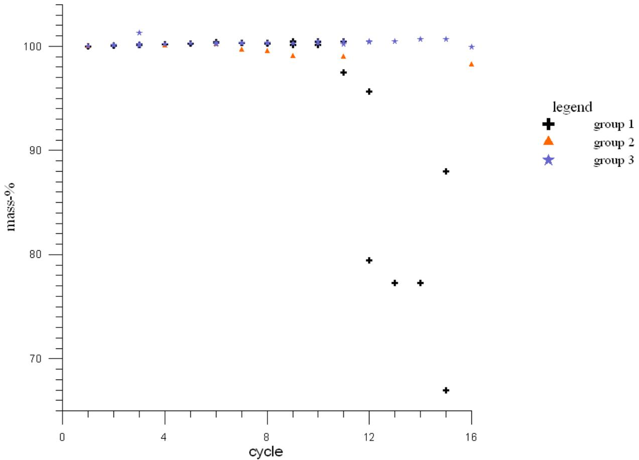
**Figure 16.** Classification of the samples in regards to their behaviour of gaining, losing or holding mass in three groups. After each cycle, the specimens were stored in a water bath for 24 hours as described in DIN EN 12370 (1999).
