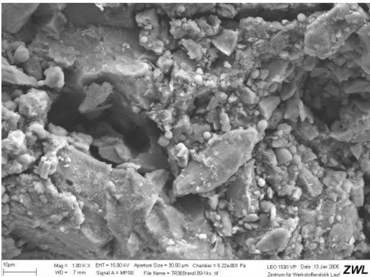
**Figure 14:** SEM-Picture. The sample was taken from the southern facade of the church and shows melt globules on the inner side of the scale. They derive from the melting of the silicates during the burning of the church.
