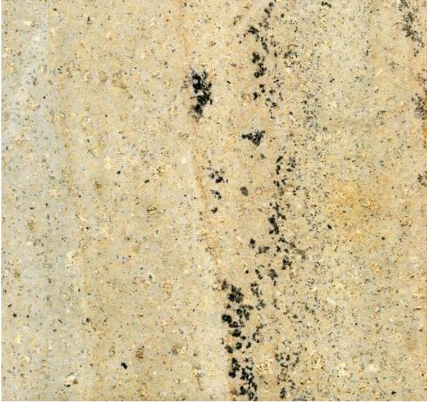
**Figure 6.** Slab of a typical yellowish-beige trachyte from the quarry (full-scale).
