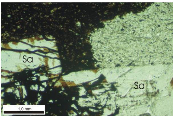
**Figure 8.** Sanidine-phenocrysts in a dense alkali feldspar groundmass. Mn-oxides diffused along the micro-cracks and cleavage faces of the sanidine crystals.
