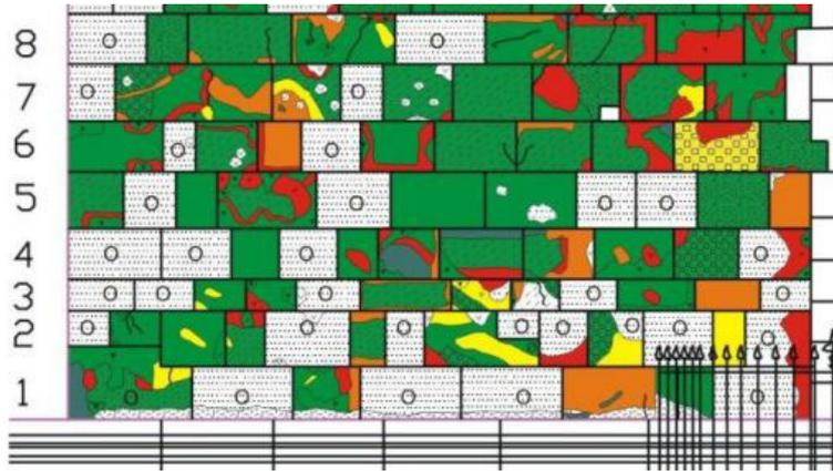
**Figure 10.** Mapping of weathering forms on the lower part of the western facade of the monastery church (cp. Figure 9). Simplified explanation of the colours: green (relief), yellow (flaking), orange (flaking due to scaling), red (scale), grass-green (soiling), white with black dots (technique of workmanship with a point chisel), black line (fissures).
