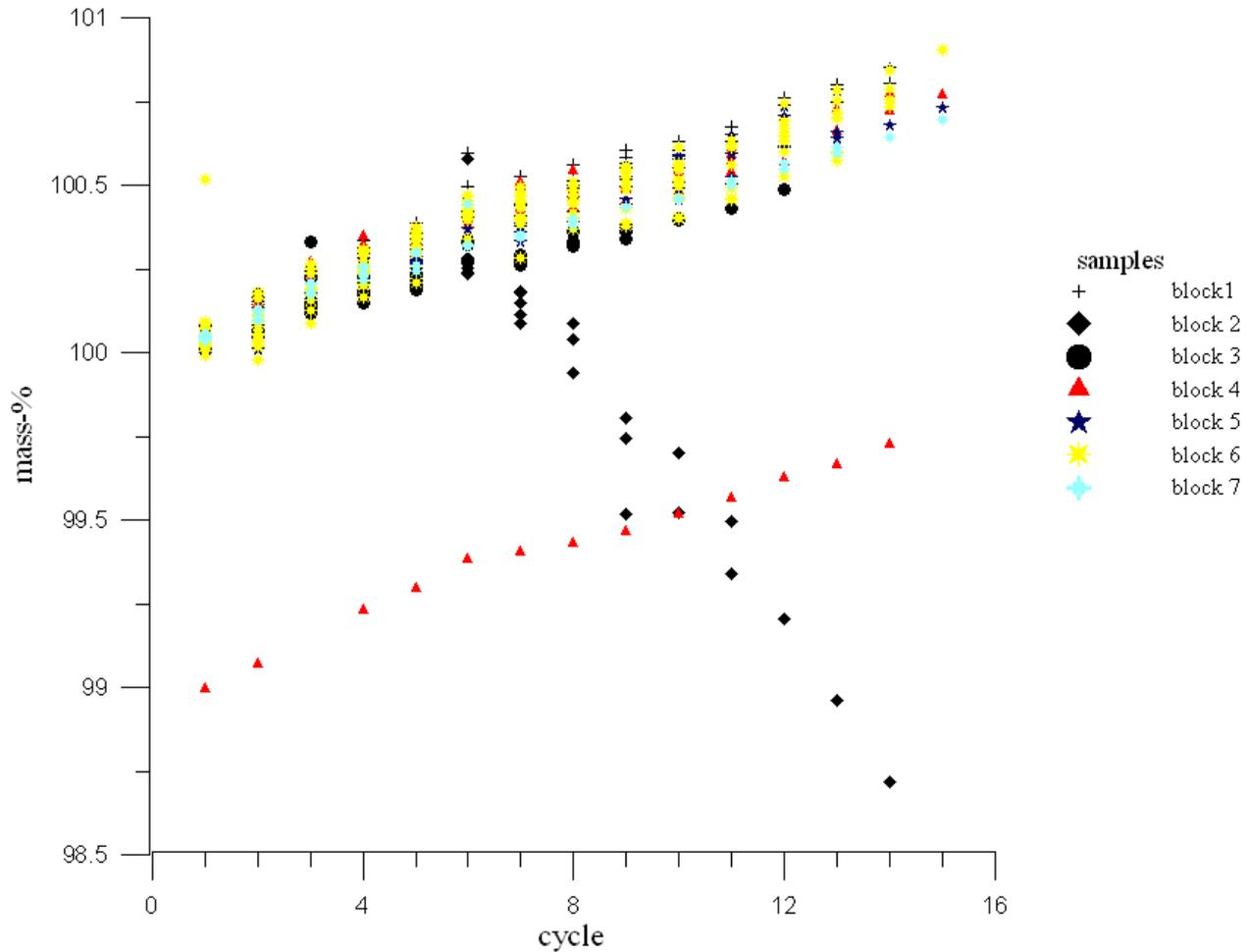
**Figure 15.** Behaviour of samples from different blocks after the cyclic salt crystallization test with sodium sulphate and before the water bath.
