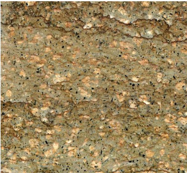
**Figure 3.** Trachite Zovonite “Calda Variegata”, Italy. Brownish variety of Trachite Zovonite “Grigia Antiacida” with its typical brown striae of limonite. The phenocrysts consists mainly of feldspar (full-scale).
