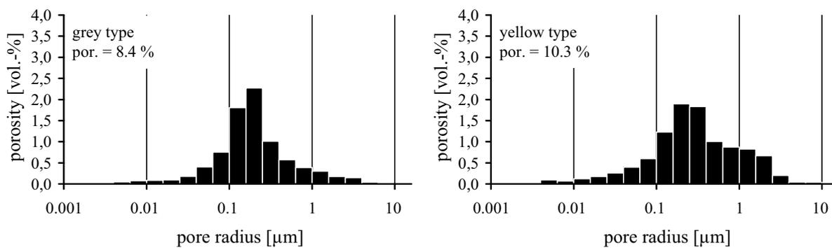
**Figure 17.** Porosities and pore size distribution of two different types of Teplá trachyte.
