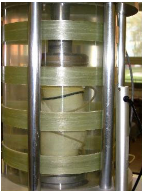
Figure 3. Destroyed sample 50 mm in cell
