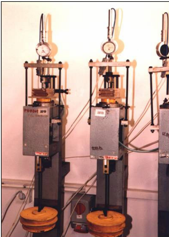
Figure 2. Oedometer loading system for consolidation of the loess samples
