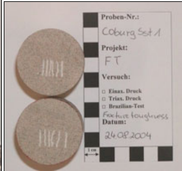
Figure 2. Tested rock specimen
