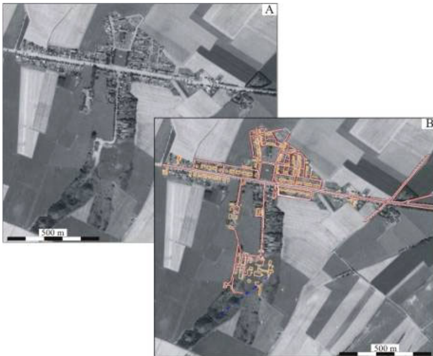
Figure 4. The digital orthophoto (upper left) is centred on the small miner’s cottage in the village of Estinnes-au-Val. Infrastructure such as the buildings and houses of the colliery, drawn on the mine plans, are given vector coordinates and superimposed perfectly on the digital orthophoto (lower right). Background image corresponds to a digital orthophoto (Copyright © National Geographic Institute).
