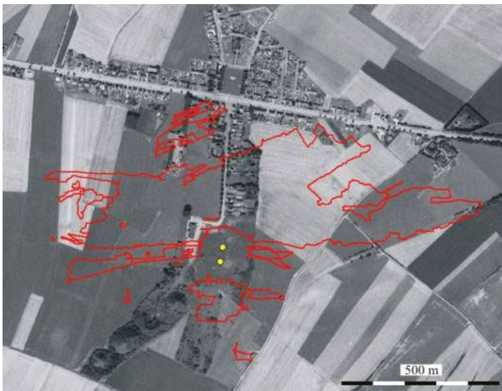
Figure 6. Limits on the surface of all the coal seams exploited between 300 and 500m deep from the two mineshafts (yellow points in the centre of the image). Background image corresponds to a digital orthophoto (Copyright © National Geographic Institute).
