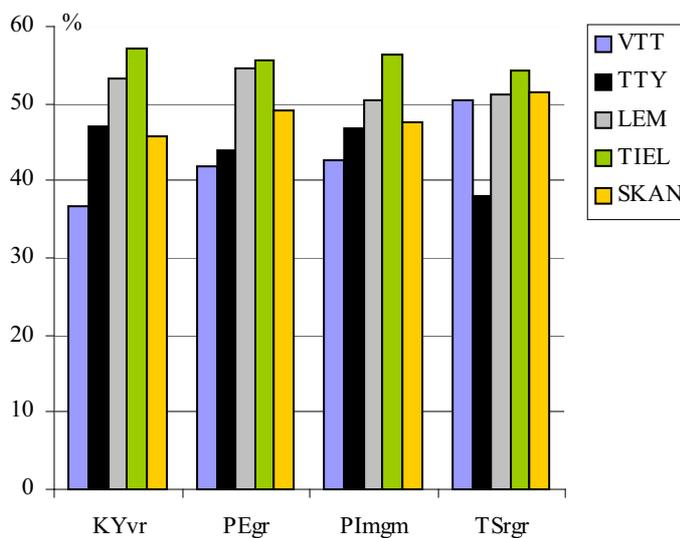
**Figure 4.** Percentages of 10/16 mm fractions after last crushing stage for each rock type in tested laboratories (measured from sieving results of flakiness index analysis). Symbols are same as in Figure 1.
