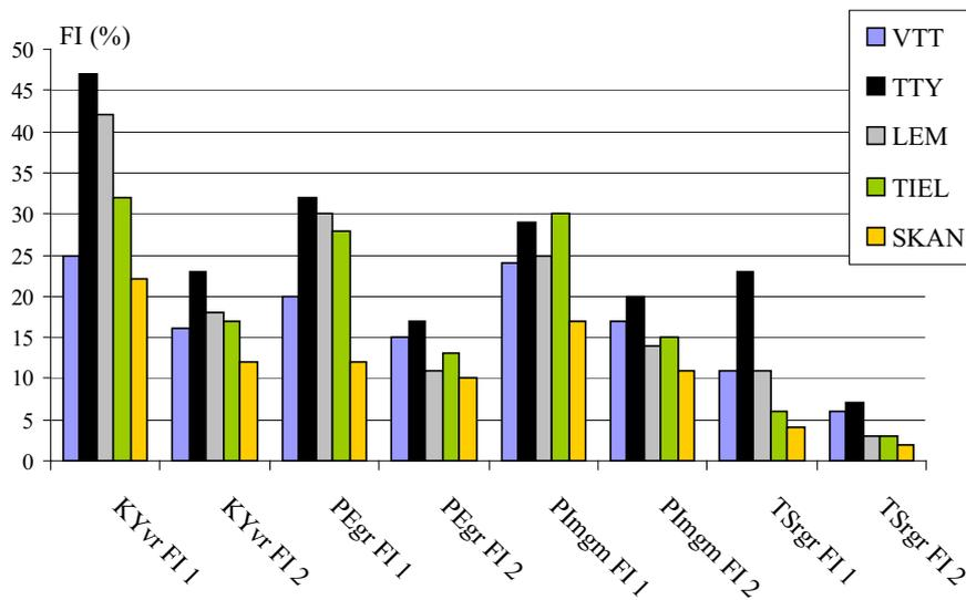
**Figure 2.** Flakiness indexes (FI) of once (1) and twice (2) crushed aggregates. Note that in VTT, TIEL, and SKAN laboratories rocks are crushed in three stages, and therefore, results of VTT, TIEL, and SKAN are from two-three times crushed aggregates. Symbols are same as in Figure 1.
