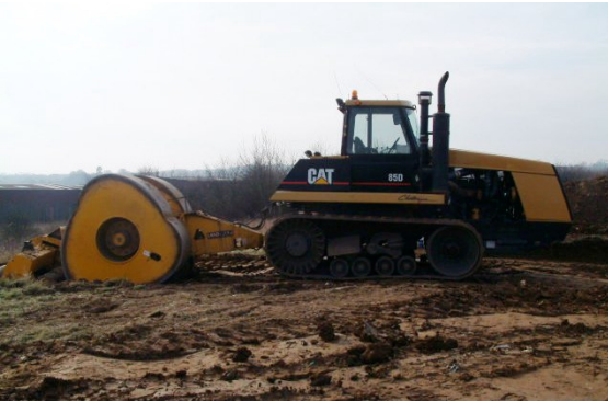
Figure 9. Photograph of Landpac HEIC plant
