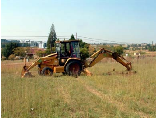
Figure 1. Backactor excavating test pit.
