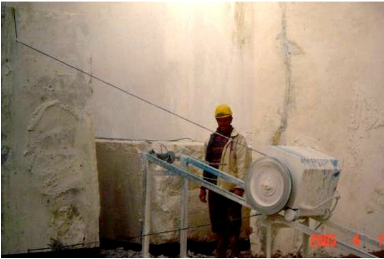
Figure 3. Diamond-wire cutter in the Quarry
