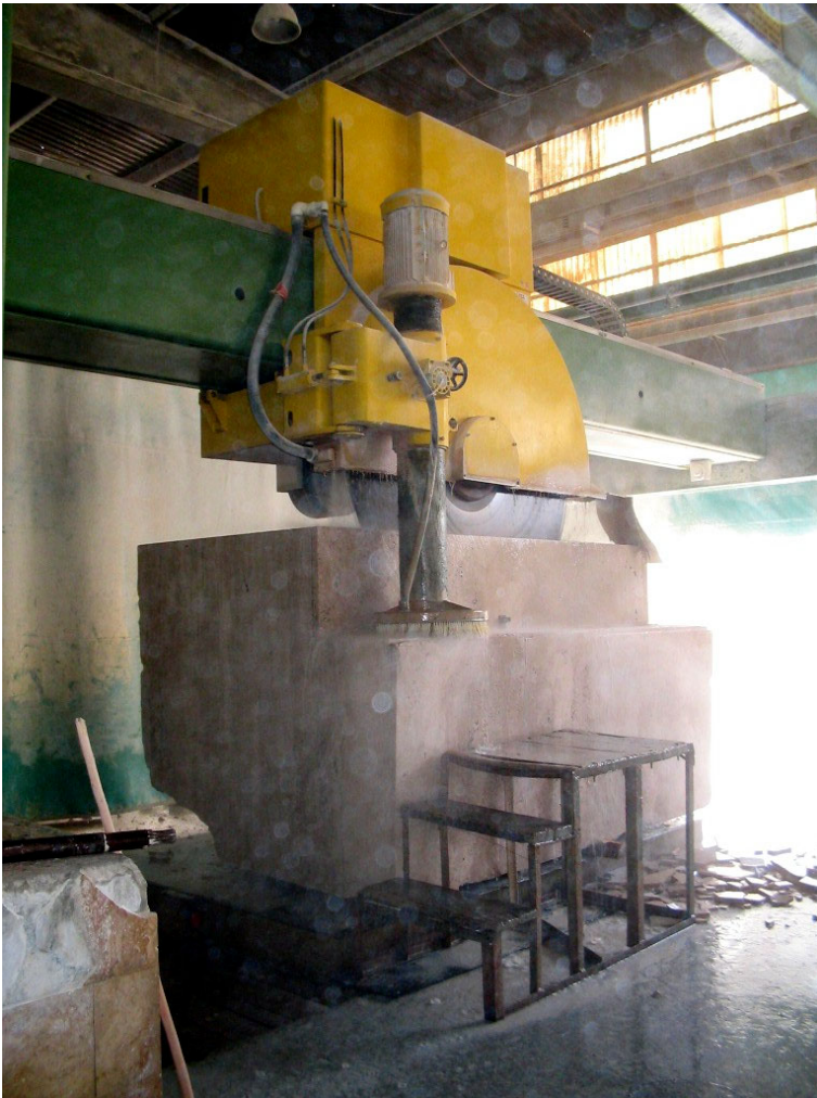
Figure 6. Large diameter ST-circular sawing machine (Courtesy of Komurcuoglu Factory)
