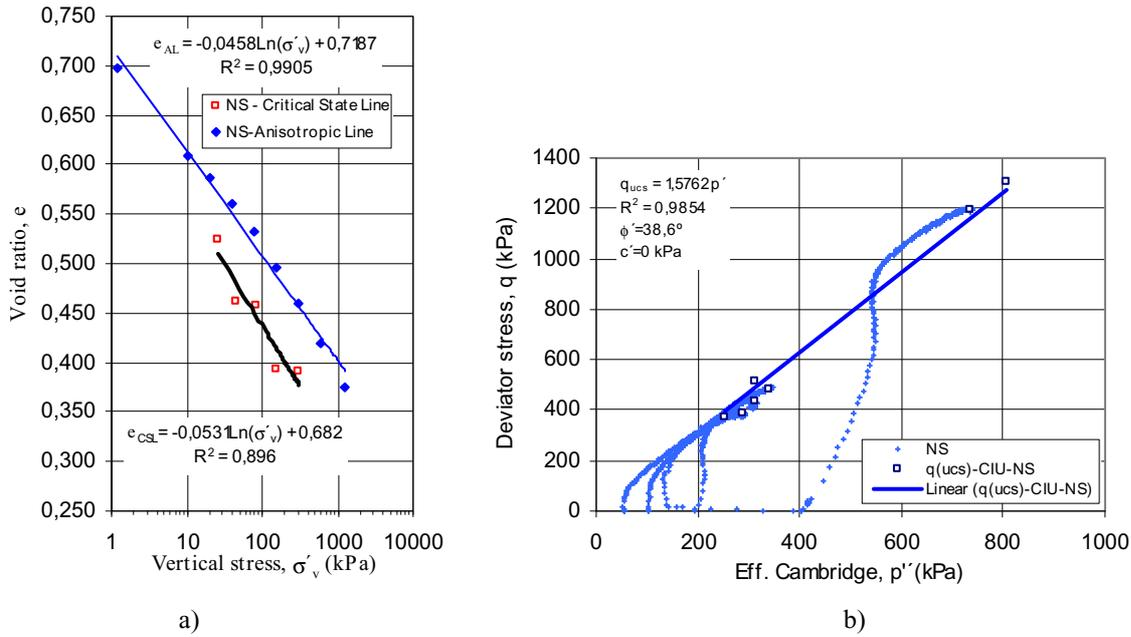
**Figure 2.** Line of the anisotropic behaviour and the critical state line of the granitic residual soil from Covilhã: a) in  $(e - \log \sigma'_v)$  space; b) in  $(q - p')$  space.
