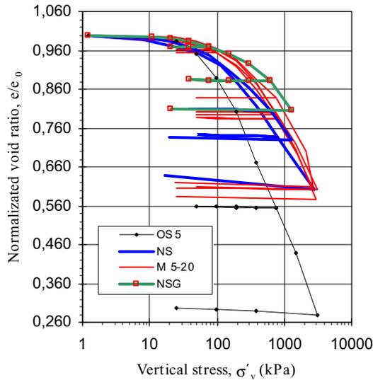
**Figure 3.** One-dimensional consolidation test results of natural (NS), artificial soil (M5-20) and soil with petrol (NSG)
