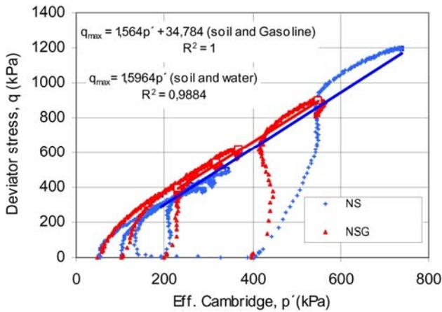
Figure 5. Undrained paths in  $q:p'$  space for the NS and NSG soil.
