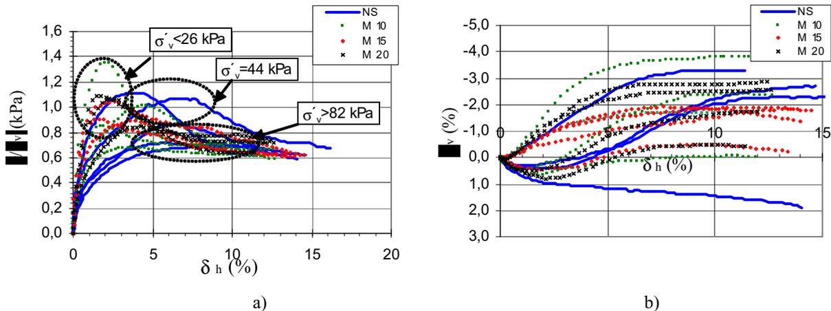
**Figure 4.** Results of direct shear tests of soil NS and soil contaminated with oil and lime: a) behaviour of normalized shear strength curves ( $\tau/\sigma'_v$ ) versus horizontal displacement ( $\delta_h$ ); b) vertical displacement curves ( $\delta_v$ ) versus horizontal displacement ( $\delta_h$ ).
