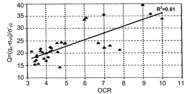
c) Relation between normalized net cone resistance and laboratory determined OCR for pliocene silty clay soils
