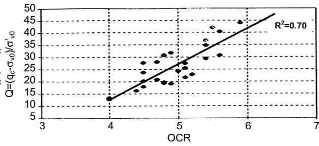
a) Relation between normalized net cone resistance and laboratory determined OCR in boulder clay soils
