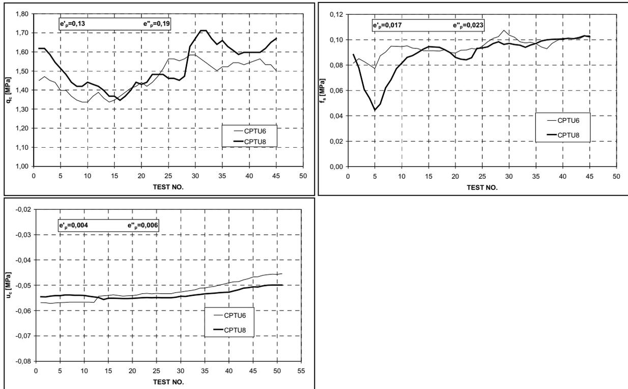
**Figure 3.** Cone penetration readings and uncertainty results
