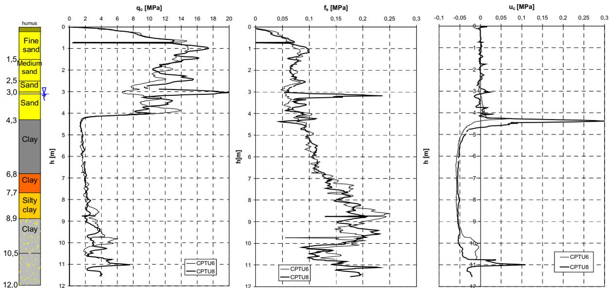
Figure 2. Cone penetration test results (CPTU)
