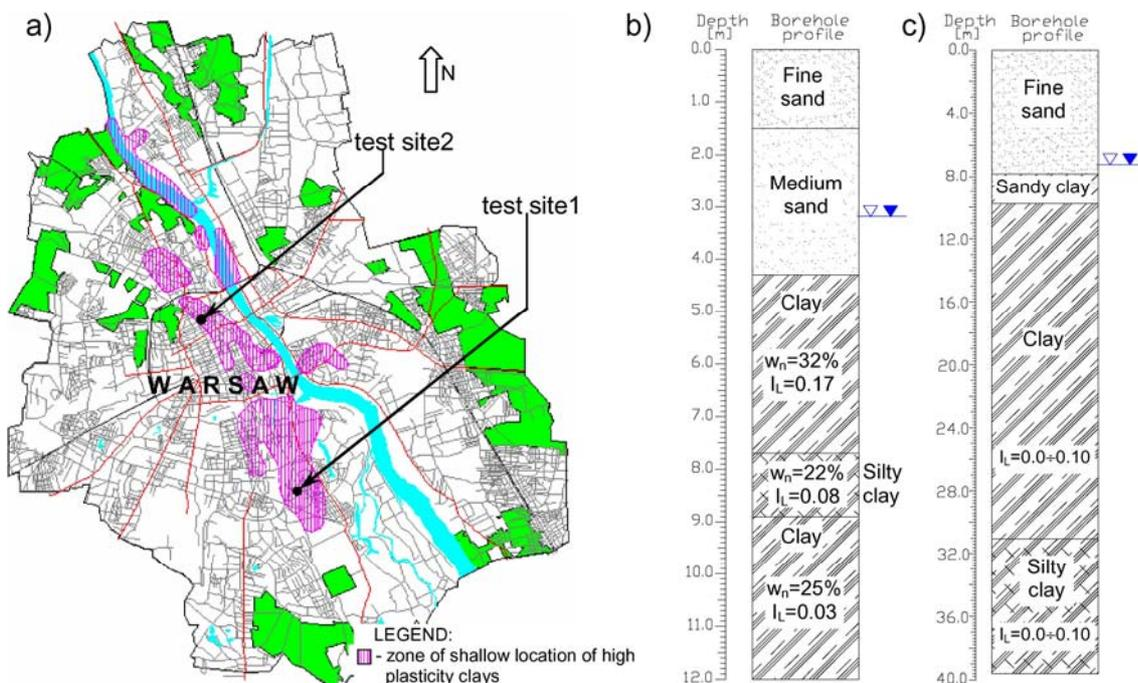
Figure 1. Test site: a) location, b) geological conditions at Stegny, c) geological conditions at Underground
