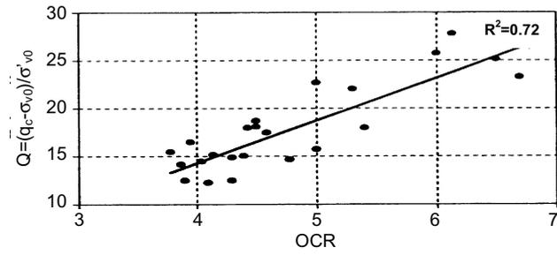
b) Relation between normalized net cone resistance and laboratory determined OCR for pliocene clay soils
