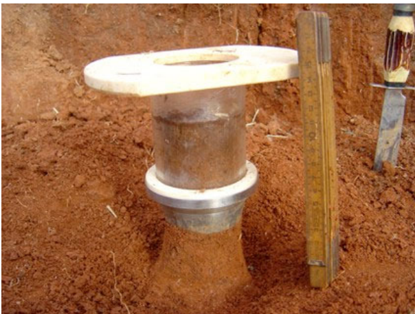
Figure 2. Collection of the undisturbed samples
