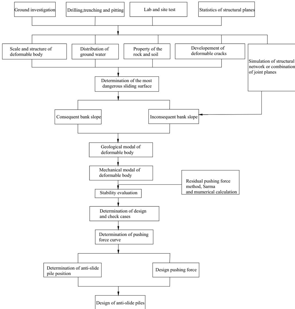
Figure 1. The research sequence of the stability evaluation and treatment of the reservoir bank.
