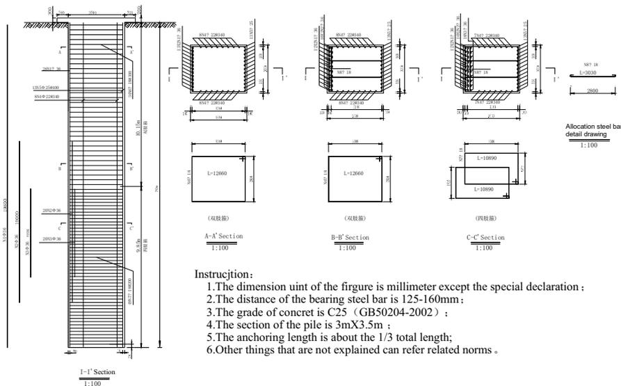
Figure 6. The structure figure of A type anti-slide pile in Archives Bureau deformable body.
