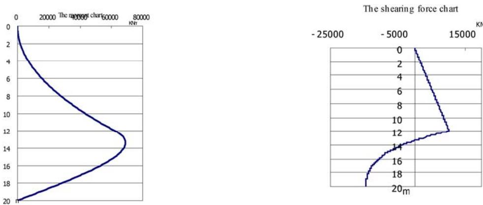
Figure 5. The moment and shearing force chart of the 8A type pile in Archives Bureau deformable body
