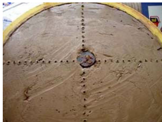
Figure 8. Open sample after measuring the electric properties between the cast iron rod and the clay
