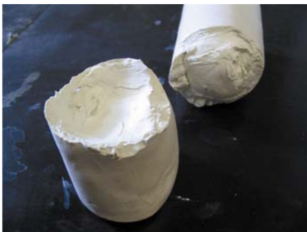
Figure 5. Concave surfaces created in the soil during one-dimensional consolidation
