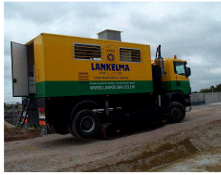
Figure 5b. Cone penetration test truck
