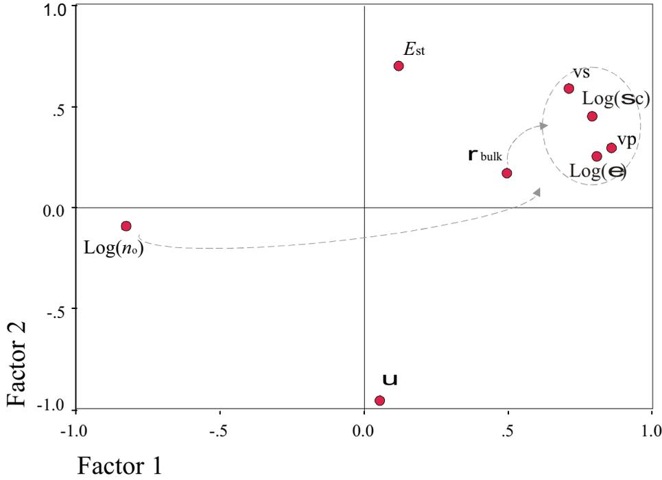
**Figure 2.** Principal component analysis with the most representative variables: P-wave velocity ( $v_p$ ), S-wave velocity ( $v_s$ ), waveform energy logarithm ( $\log(\varepsilon)$ ), density ( $\rho_{\text{bulk}}$ ), effective porosity logarithm ( $\log(n_o)$ ), compressive strength logarithm ( $\log(\sigma_c)$ ), Young static elasticity modulus ( $E_{st}$ ) and Poisson's ratio ( $\nu$ ).
