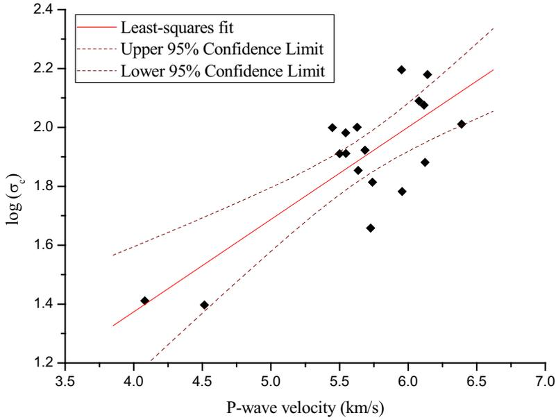
**Figure 3.** Relationship between logarithm of uniaxial compressive strength ( $\log(\sigma_c)$ ) and P-wave velocity.
