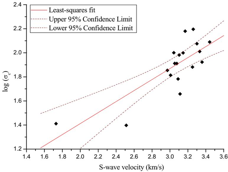
**Figure 4.** Relationship between logarithm of uniaxial compressive strength ( $\log(\sigma_c)$ ) and S-wave velocity.
