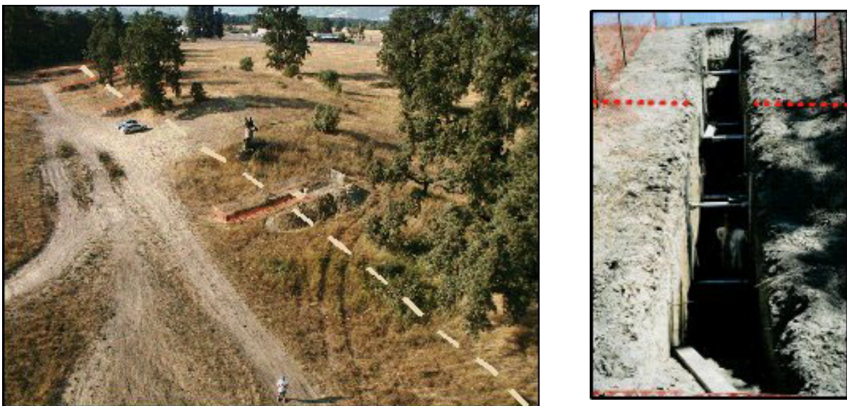
Figure 5. Fault trench investigations along the Maacama fault, Mendocino County, Northern California. Main fault trace marked by dashed lines. Multiple trenches provide a picture of along-strike changes in fault rupture style.
