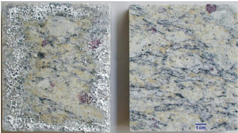
Figure 6. Crystallization of salts at the borders of test specimen, preferentially on biotite sites (control specimen on the right).
