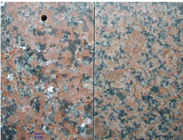
Figure 2. Formation of salt (in white) in surface microcracks and locally on biotite after exposure to sulphur dioxide (control specimen on the right).
