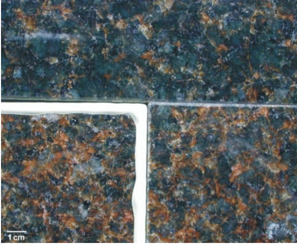
Figure 3. Increasing of pre-existent oxidation after exposition to salt mist (above: control specimen).
