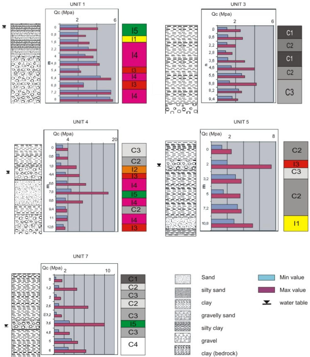
Figure 4. Typical stratigraphical and geotechnical profiles of the different engineering geological units.
