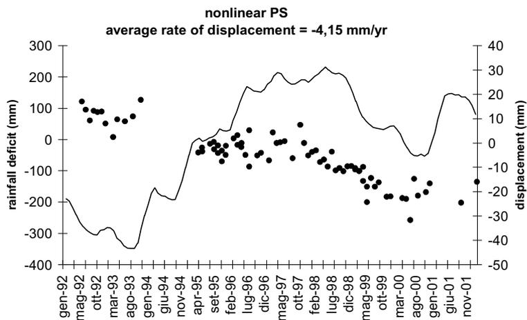
Figure 9. Rainfall deficit vs. PS displacement series (sub-unit “silty clay with layer of sand”).
