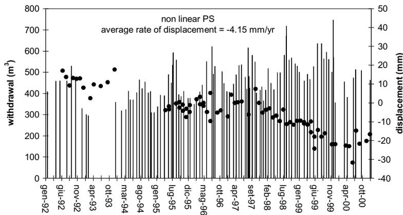
Figure 10. Daily withdrawal vs. PS displacement series (sub-unit “silty clay with layer of sand”).
