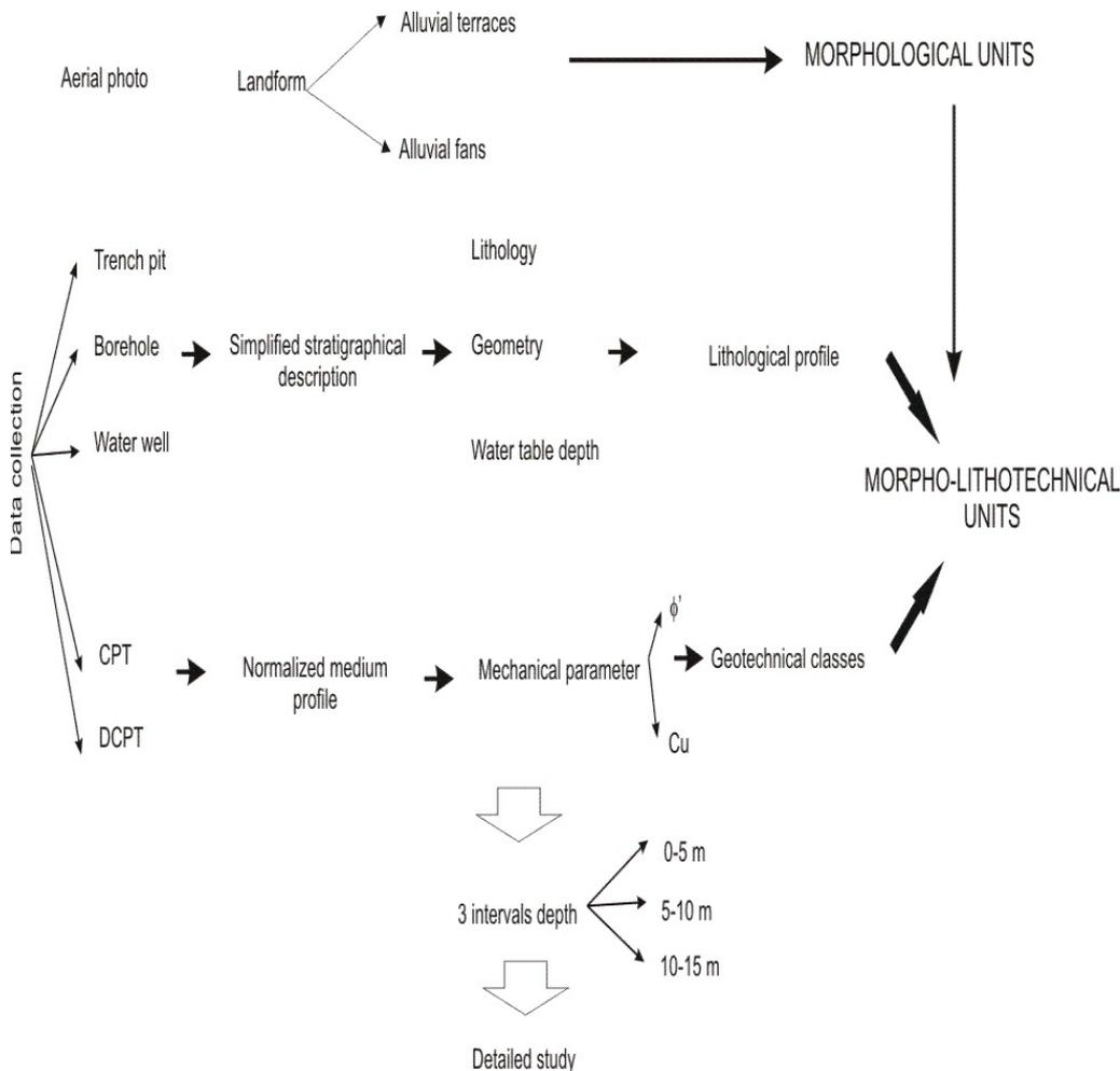
**Figure 2.** Steps to identify the engineering geological terrain units.
