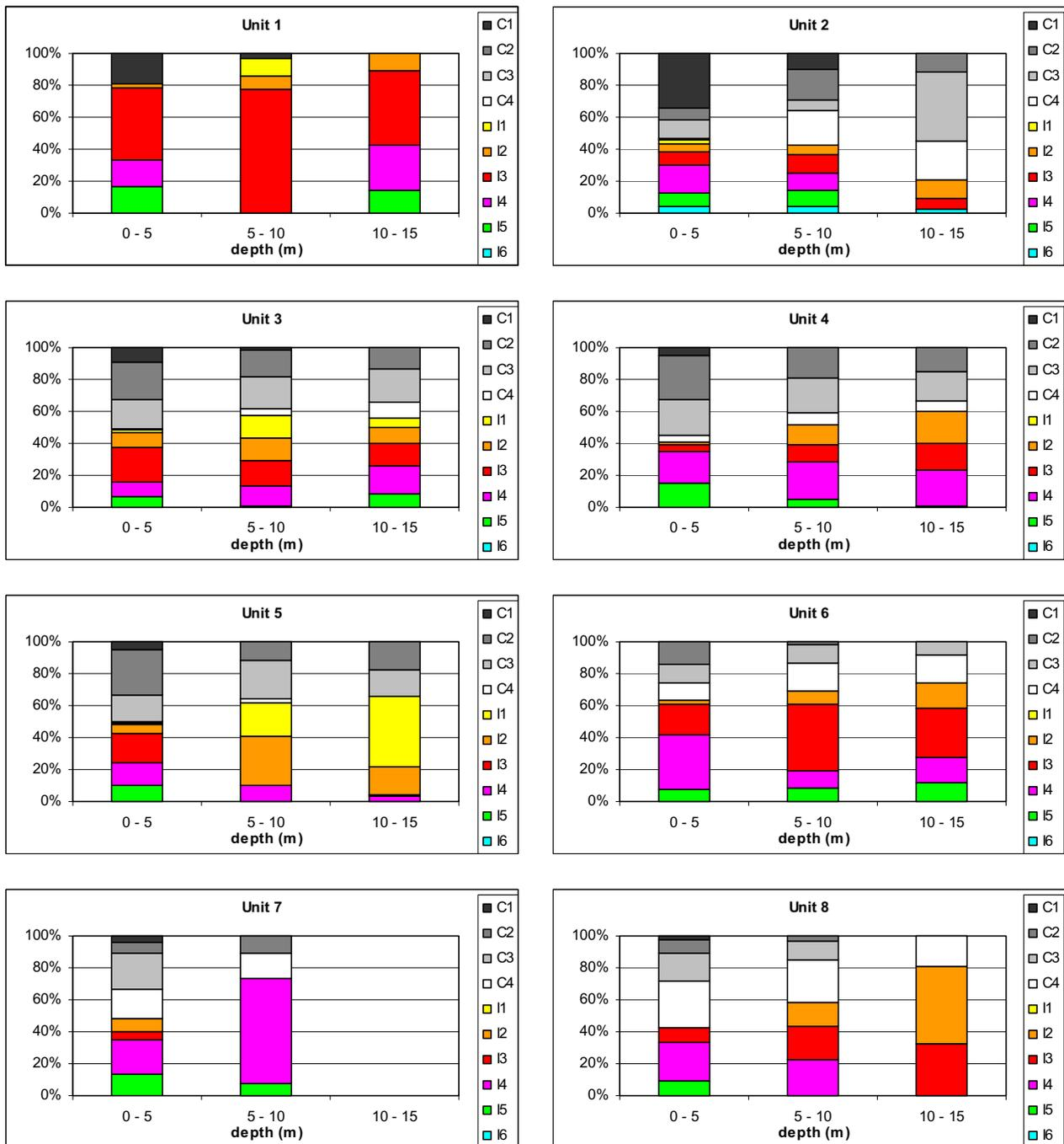
**Figure 5.** Thickness (%) of the different geotechnical horizons over different depth intervals.
