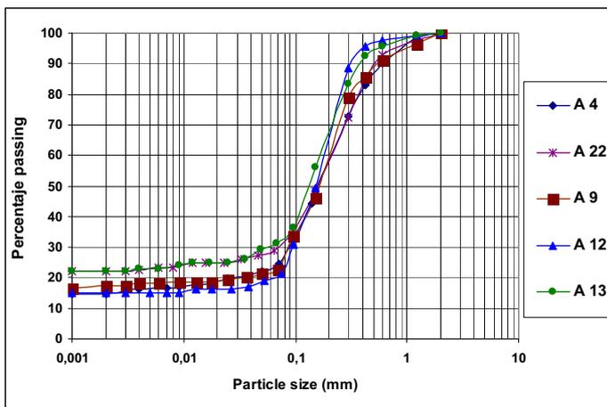
Figure 6. Size particle curves for unconsolidated materials of the Unit II.
