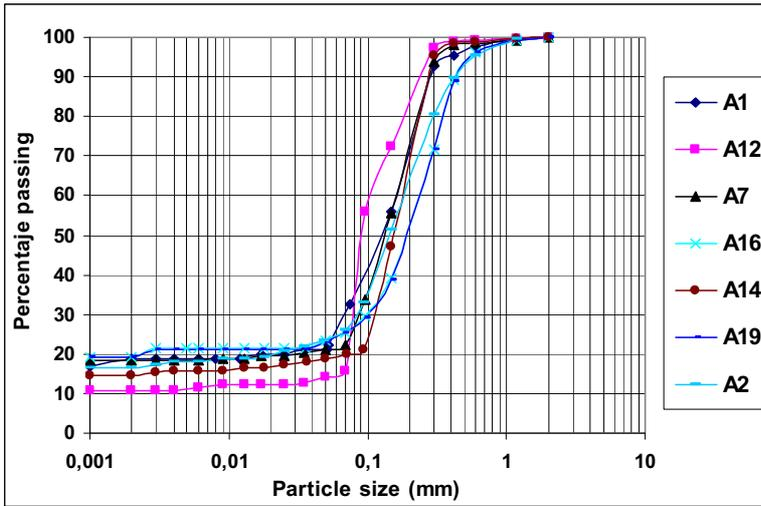
Figure 10. Size particle curves of the unconsolidated material - Clayed sand layer of the subunit 2-Unit III.
