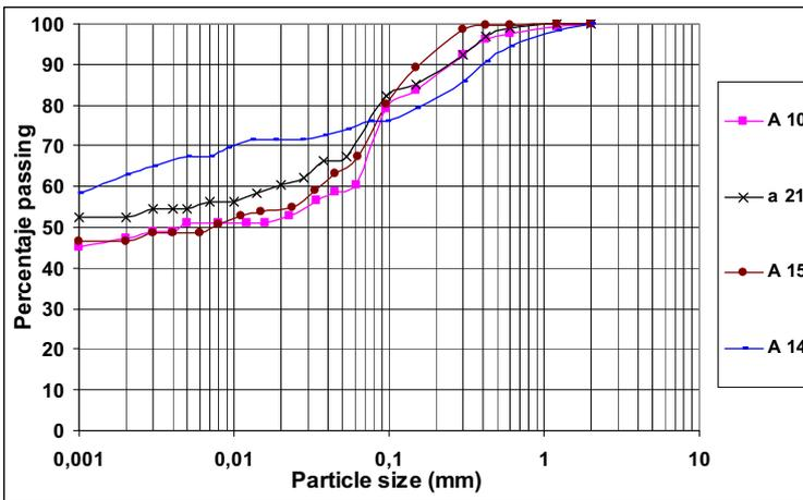
Figure 14. Size particle curves of the unconsolidated material of the subunit 4 of the Unit III.
