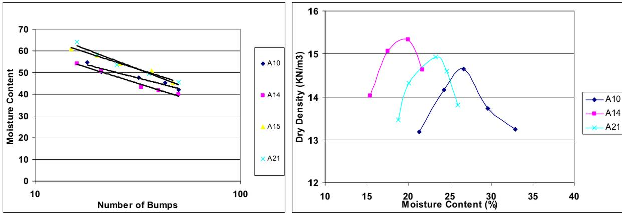
Figure 15. (A) Liquid limit results and graph for unconsolidated material- clay layer, Subunit 4 - Unit III and (B) Compaction curves for unconsolidated materials - clay layer, Subunit 4 - Unit III.
