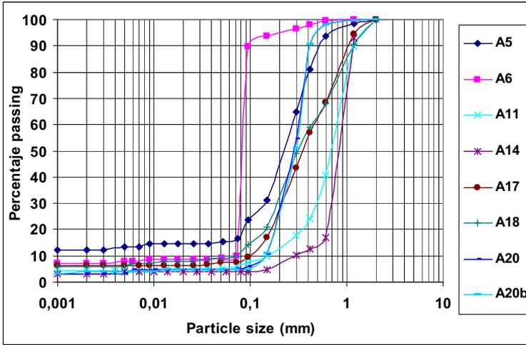
Figure 12. Size particle curves of the unconsolidated material of the subunit 3 of the Unit III.
