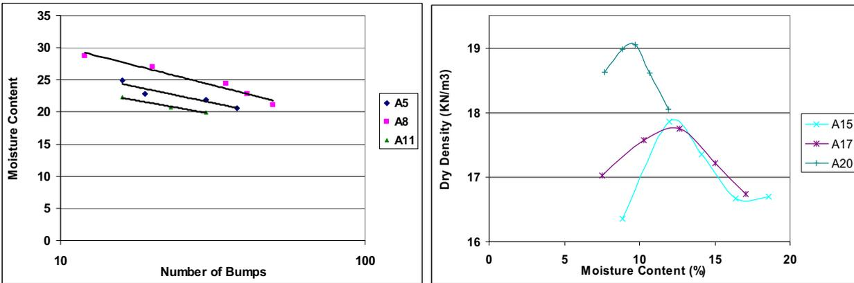
Figure 13. (A) Liquid limit results and graph for unconsolidated material - Non-concretionary accumulation of iron sand layer, Subunit 3 - Unit III and (B) Compaction curves for unconsolidated materials – Non-concretionary accumulation of iron sand layer, Subunit 3 - Unit III.
