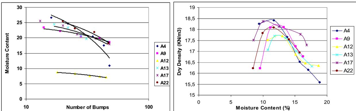
Figure 7. (A) Liquid limit results and graph for unconsolidated materials of the Unit II and (B) Compaction curves for unconsolidated materials of the Unit II.
