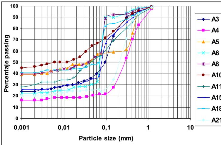
**Figure 8.** Size particle curves for unconsolidated material of the subunit 1- Unit III.
