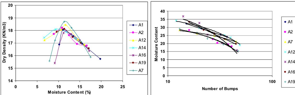
Figure11. (A) Compaction curves for unconsolidated materials – Clayed sand layer, Subunit 2 - Unit III and (B) Liquid limit results and graph for unconsolidated materials – Clayed sand layer, Subunit 2 - Unit III.
