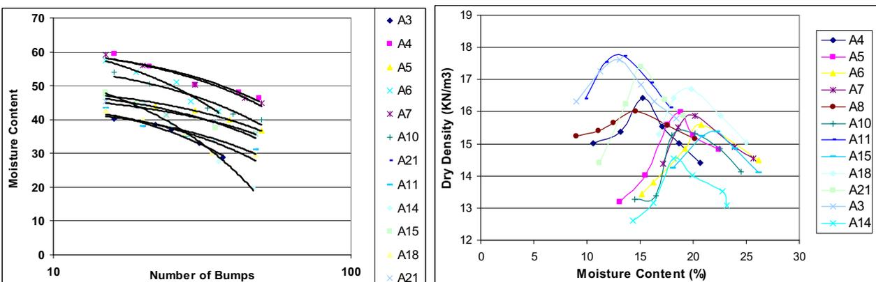
**Figure 9.** (A) Liquid limit results and graph for unconsolidated material - Concretionary layers, Subunit 1 - Unit III and (B) Compaction curves for unconsolidated materials - Concretionary layer, Subunit 1 - Unit III.
