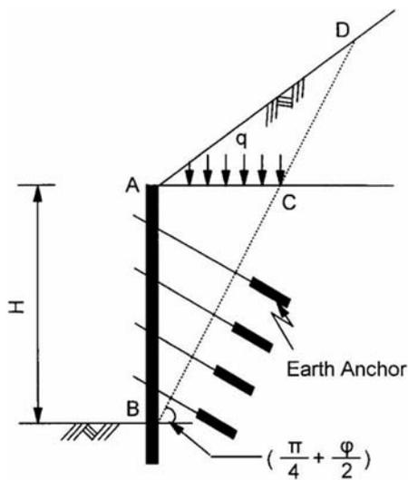
Figure 10. Earth pressure calculation method
