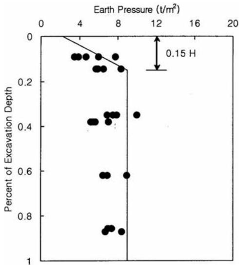
Figure 8. The measured earth pressure
