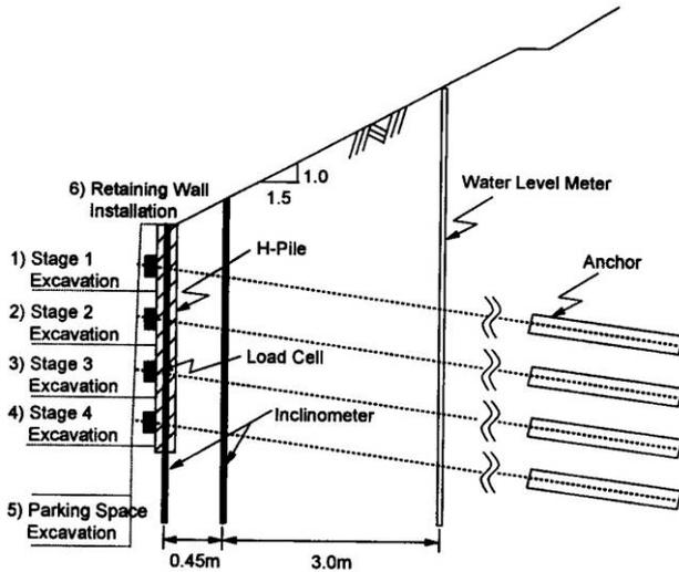
Figure 4. Cross-sectional view of instrumentation system
