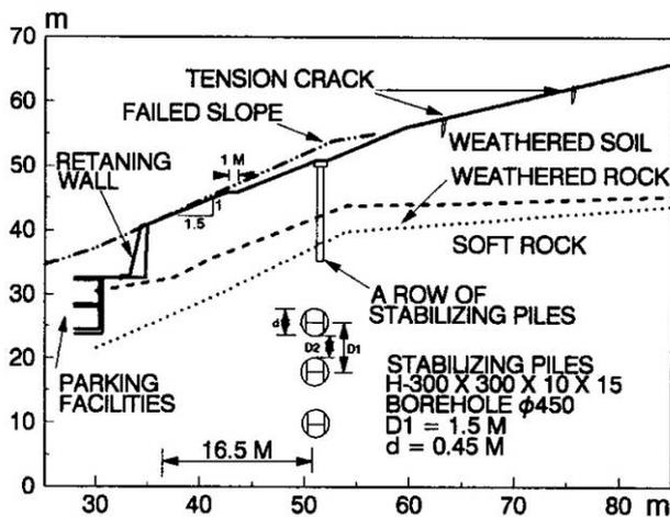
Figure 2. Layout of slope stabilization (section A-A)
