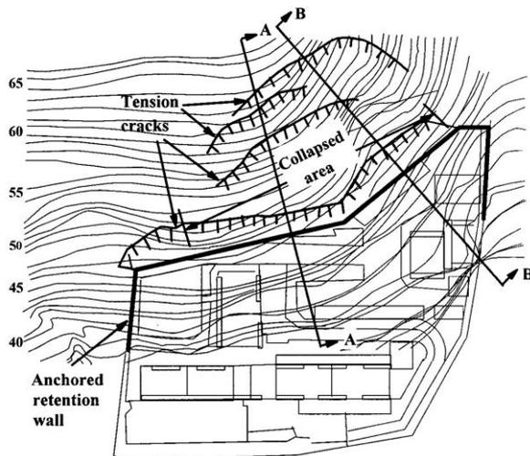
Figure 1. Plan view of landslide outline
