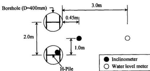
Figure 5. Plan view of instrumentation system
