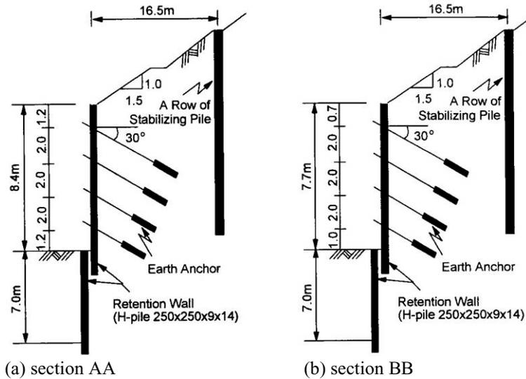
Figure 3. Anchored retention walls installed in cut slopes
