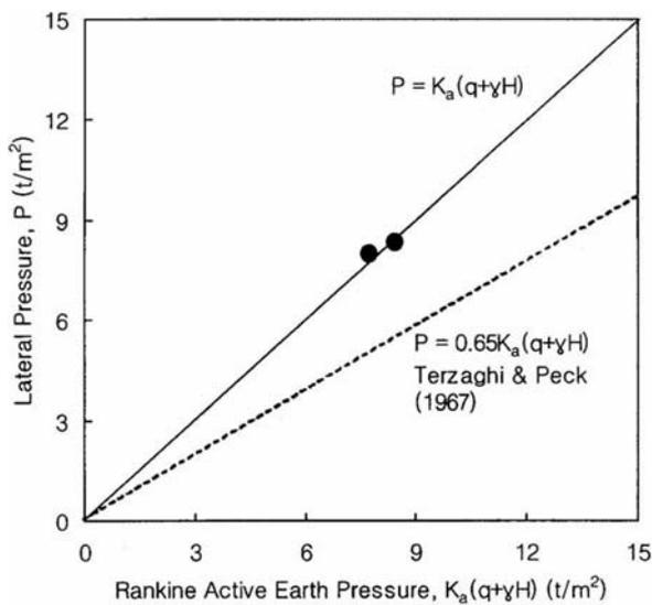
Figure 11. Comparison with the empirical earth pressure
