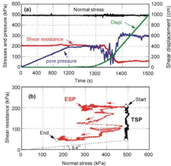
**Figure 19.** Results of a ring-shear test on a sample from the Azue landslide source area. (a) Time-series data for normal stress, shear resistance, pore-water pressure and shear displacement; (b) stress path (ESP: Effective Stress Path; TSP: Total Stress Path) ( $B_d = 0.96$ ,  $e = 0.425$ )
