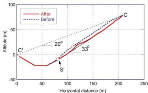
**Figure 14.** Longitude section of the Kamagatani landslide (S' is sample point; the pre-failure topography was obtained from neighbouring slope)
