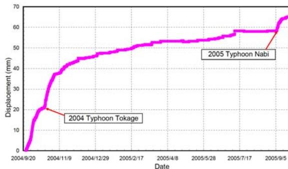
**Figure 11.** Monitored displacement from Sept. 22, 2004 to Sept. 26, 2005 on the back crack
