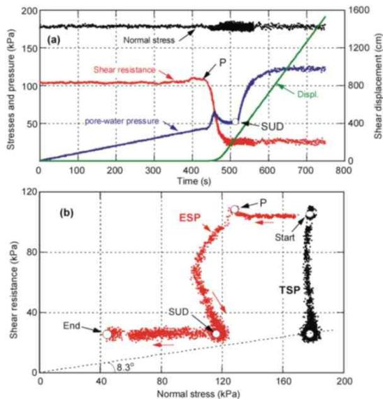
**Figure 20.** Results of a ring shear test on a sample from the Kamagatani landslide source area. (a) Time-series data for normal stress, shear resistance, pore-water pressure and shear displacement; (b) stress path (ESP: Effective Stress Path; TSP: Total Stress Path) ( $B_d = 0.97$ ,  $e = 0.513$ )
