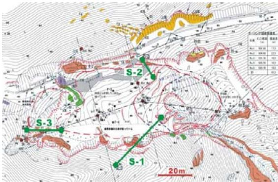
Figure 16. Plan of the source area of Shiraiishi landslide, and the unstable block after the landslide event as well as the locations of extensometers
