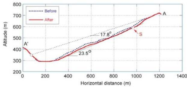
**Figure 9.** Longitudinal section of the Azue landslide (A-A' in Figure 7; S is sample point)
