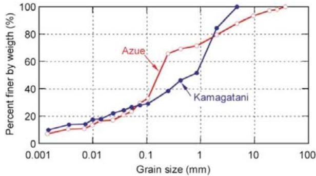
**Figure 18.** Grain-size distributions of samples from the Azue and Kamagatani landslides (after removal of the >2 mm size fraction)
