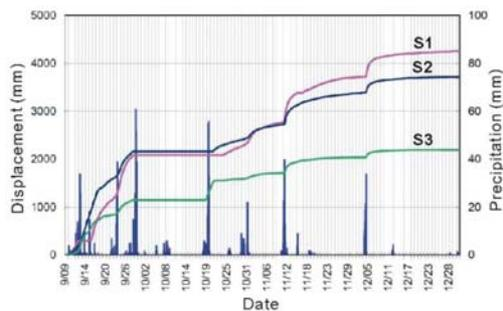
Figure 17. Monitored rain precipitation and displacement
