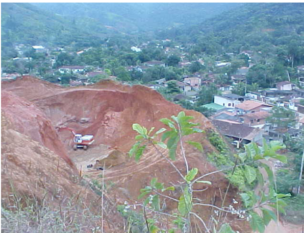
Figure 7. Example of an environmentally degraded site. Active mineral exploitation of residual soil (licensed). Hazardous area due to declivity, ground instability and close proximity of housing areas.
