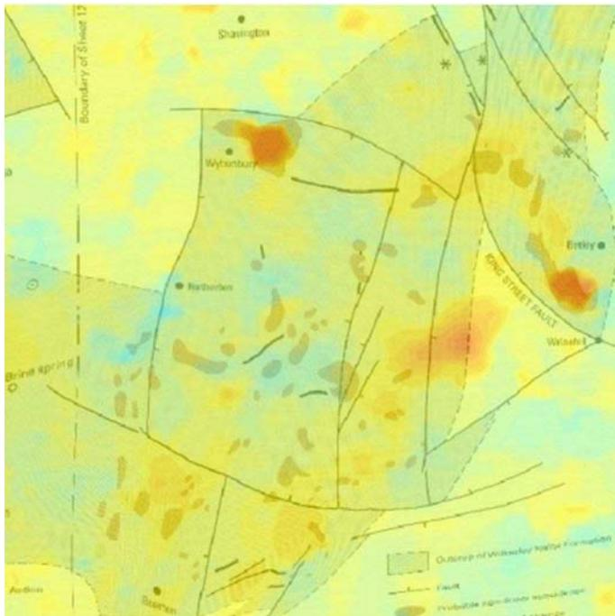
**Figure 10.** Wilkesley Halite Formation (grey polygons) and areas of probable non-linear subsidence (brown areas) overlain by the interpolated PS data.
