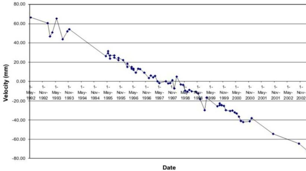
**Figure 9.** PSInSAR derived velocity for the point nearest to the Crowcrofts fault and the levelling data gathered by Donnelly (1994). The time period runs from May 1992 to November 2002. Horizontal lines are scaled 20 mm apart.
