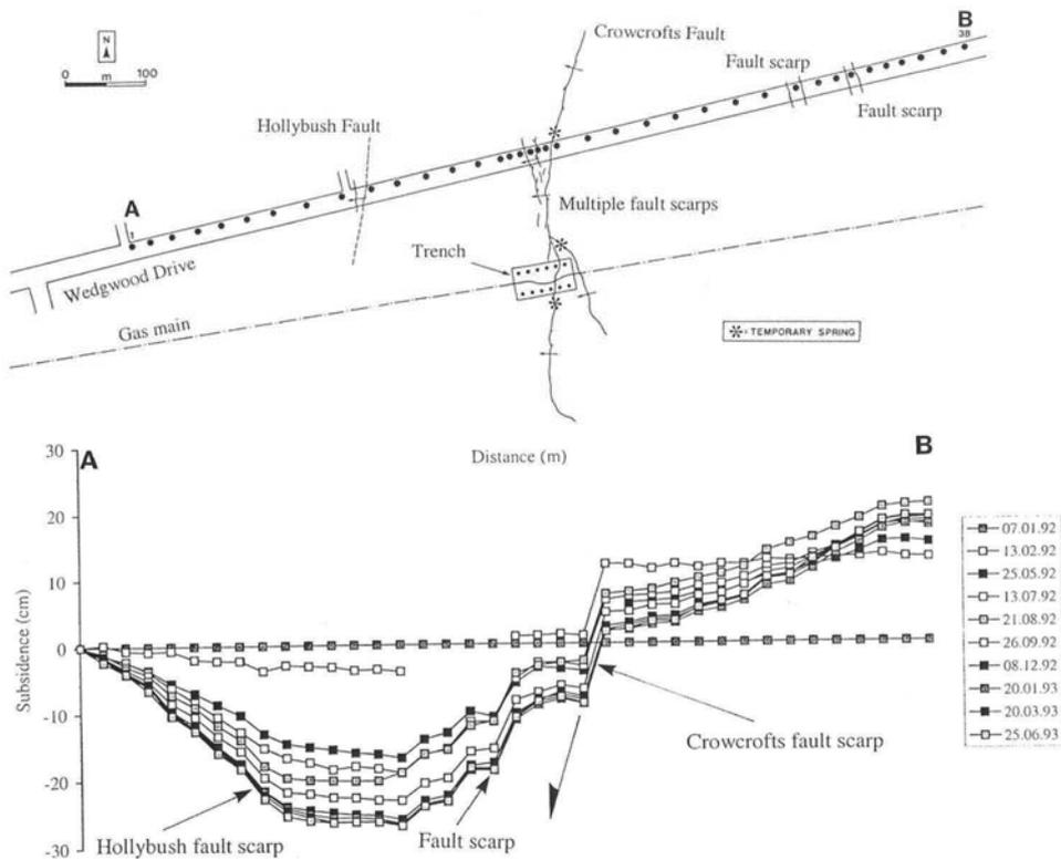
**Figure 8.** The levelling traverse along Wedgwood Drive and motion associated with the fault.
