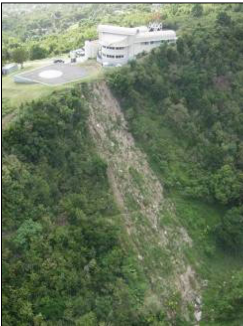
Figure 7. The Montserrat Volcano Observatory landslide; a complex debris slide earthflow with a component of rotational slip (source: Montserrat Volcano Observatory & British Geological Survey).
