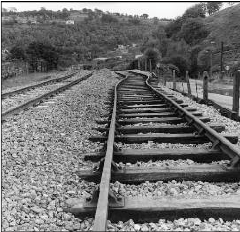
Figure 7. Reactivation of the Kilkenny Fault, South Wales, UK causing severe damage (compression) and buckling to the Cardiff to Taff Merthyr railway tracks.
