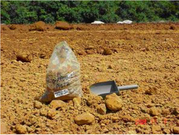
Figure 5. Lateritic concretion used as sub-base and base of track of the aerodrome.
