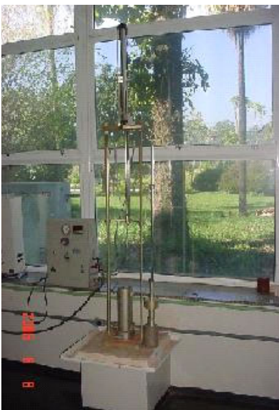
Figure 6. Pneumatic MCV-ITA Equipment.
