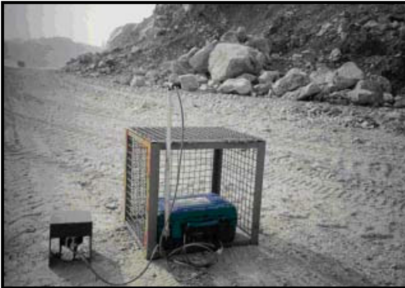
Figure 4. Digital recordings for ground vibration and air blast during bench blasting.
